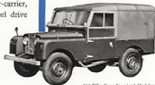
86" Wheelbase Standard Model with detachable hood and side screens.
