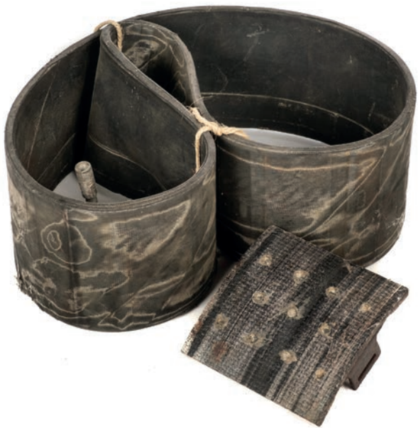
19* Avro Lancaster. A WWII brake shoe and inflatable main brake bellows from Avro Lancaster NX611 'Just Jane', the brake shoe 13 x 13cm, the inflatable main brake measuring 14cm wide, corrosion to both Provenance: Lincolnshire Heritage Museum.
