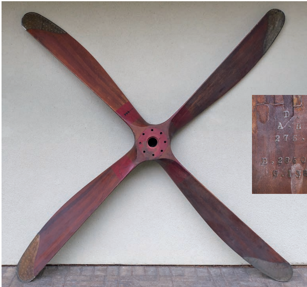
100* Propeller. A fine WWI four-blade propeller from an Airco DH4, the laminated mahogany blades sheathed in brass, retaining original red factory paint, the boss stamped D.H.4., A.B. 6861, 275 H.P. P.R., R.H., D.2850. P. 3600, G. 136. NO. 61, additionally stamped 138 No 61 The Airco DH4 was a British two-seat biplane day bomber used extensively during WWI. It was designed by Geoffrey de Havilland and was used for both day bombing and reconnaissance missions. Postwar service saw the DH4 used as a mailplane and an early commercial passenger airplane to Europe. (1) £2,000 - £3,000
