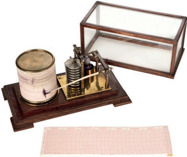
319* Barograph. A 1920s brass barograph by Ross of London, presented in an oak and glass display case, 15cm high x 31cm wide x 18cm deep
