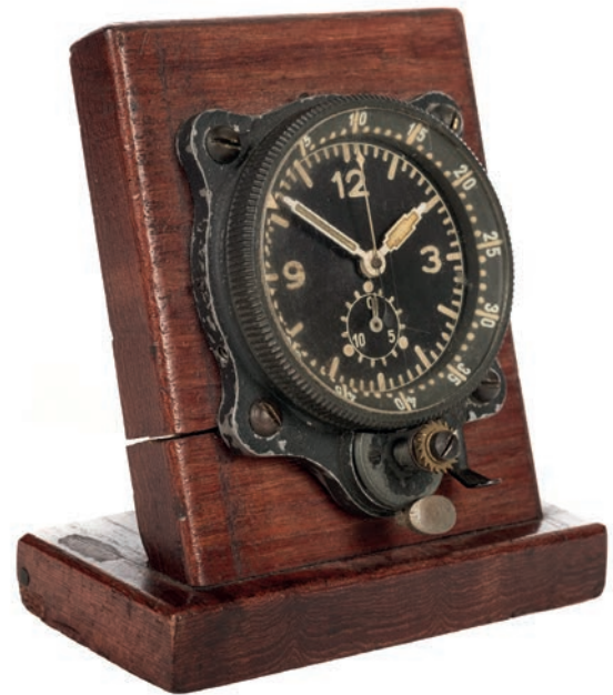
80* Luftwaffe. WWII Junghans Borduhr Cockpit Clock, numbered 860604, black dial with illuminated hands and Arabic numerals, the movement stamped J30 BZ', 50mm diameter dial, in working condition and mounted in on a wooden display stand (1)
