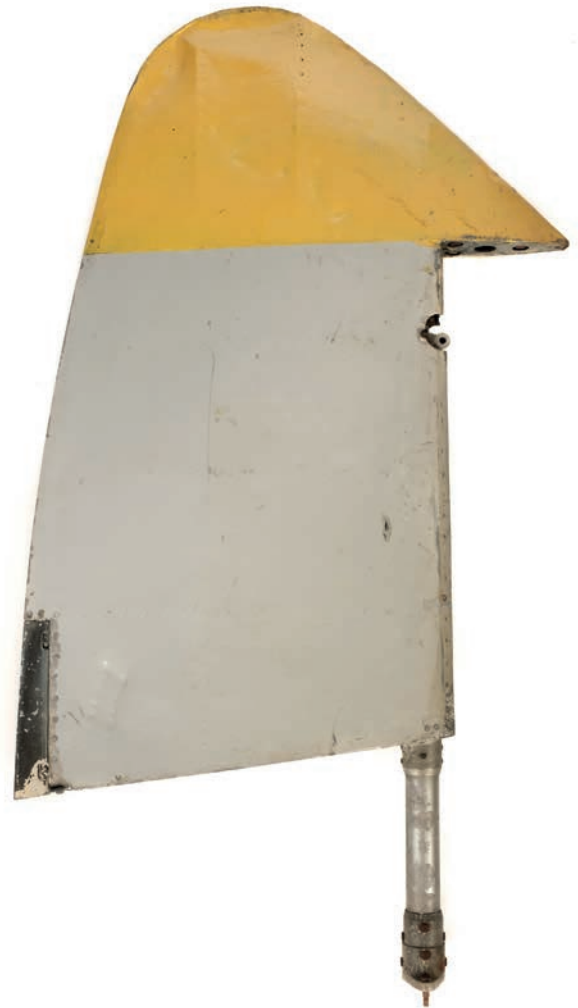
56* De Havilland. DH113 Vampire jet fighter rear boom rudder, aluminium finished in grey with yellow tip, data plate on the edge stamped 'D.H. 113, Serial No DHB 2133, Drg No 13TR 1 A/3, Issue No 16, Insp DHB 99, Mods 11-Y-7, 3621, 3628, 21/1/64', overall length 113cm. From T11 Vampire XD534, formerly owned by the vendor.
