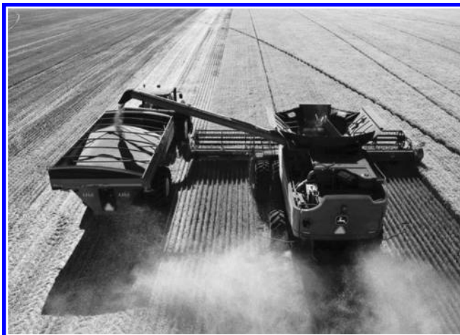
FIGURE 5.9 John Deere’s Machine Sync that can synchronize the operation of combines and tractors with grain carts for “on-the-go” harvesting. (Photo courtesy of Deere & Company.)
