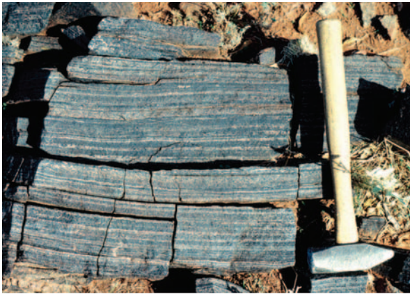
FIGURE 5 Layered quartz-tourmaline tourmalinite in the Broken Hill district, Australia, from the same stratigraphic level as the main Pb-Zn-Ag lodes
