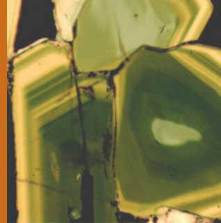
Zoned tourmaline from the Ore Knob VMS deposit, North Carolina, USA. The matrix (black) is chalcopyrite.
