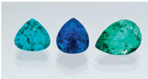
FIGURE 4 Faceted elbaite stones from Paraíba, Brazil (2.59–3.68 ct; the stone on the left is about 6 mm tall). These stones owe their intense, “neon” blue colors to the influence of \text{Cu}^{2+} in the tourmaline structure. In some cases, \text{Cu}^{2+} in combination with other cations modifies the resulting colors. © GEMOLOGICAL INSTITUTE OF AMERICAN. PHOTO BY ROBERT WELDON. REPRINTED BY PERMISSION
