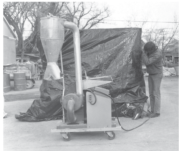
Figure 4 —Hammermill used to remove seed appendages.
