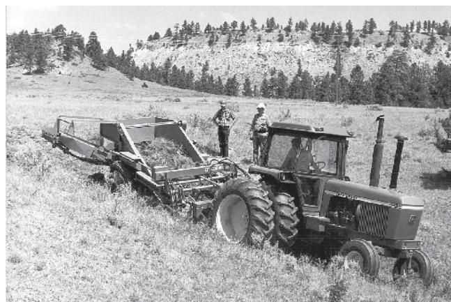
Figure 13 —“Sprigger” used to collect rhizomatous planting stock.
