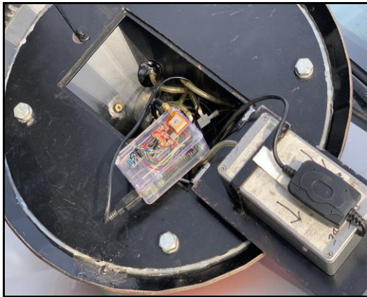
Figure 7: PACRITEX probe showing 4.7-mm steel plating and internal electronic data-logging equipment.
