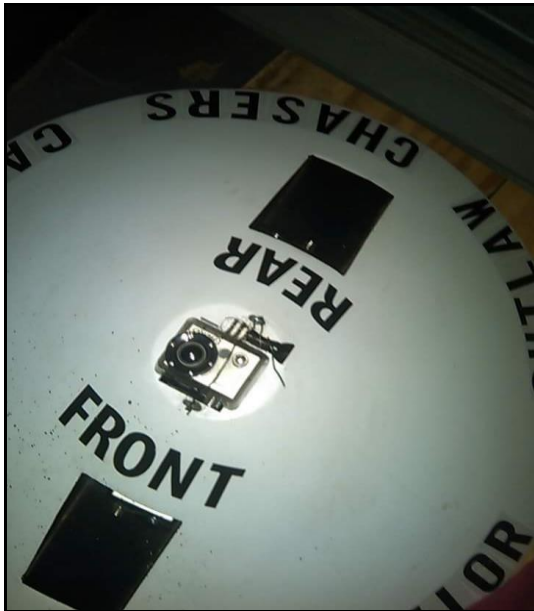
Figure 9: PACRITEX video probe with flat-top design, shadow boxes, and video cameras attached test results. Simply stated, a probe would need to be placed inside the tornado core to see if it would survive.
