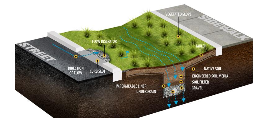
Specialized vegetated channels designed to slow stormwater runoff, promote infiltration, trap sediment, and treat pollutants.
