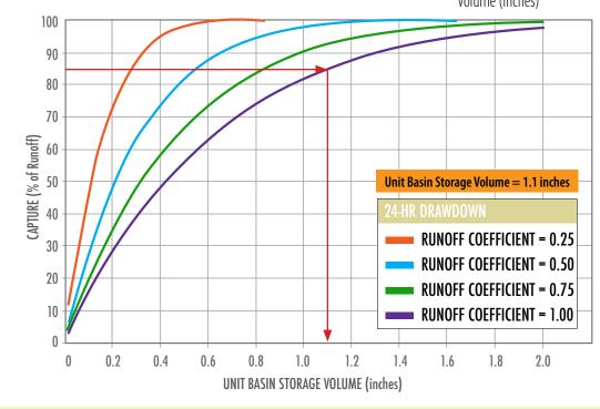
• Calculate the design Volume necessary to capture the 85<sup>th</sup> percentile runoff:
