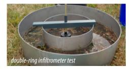
The permeable pavers / pavement selected should have an infiltration rate greater than or equal to fdesign. If that cannot be achieved, revise fdesion to match the maximum allowable infiltration rate of the pavers / pavement selected.
