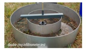
The double-ring Infiltrometer and well permeameter tests are preferred, but whatever test is used must be performed at each location and elevation where the Green Street LID Application is proposed. Multiple tests at each site are recommended.
