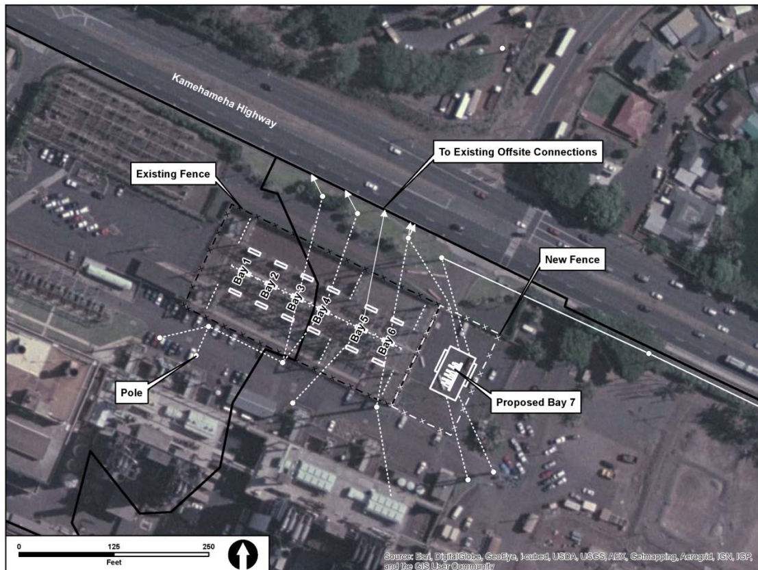
Figure 3.13 Conceptual Layout of 138 kV Substation Retrofit Project
