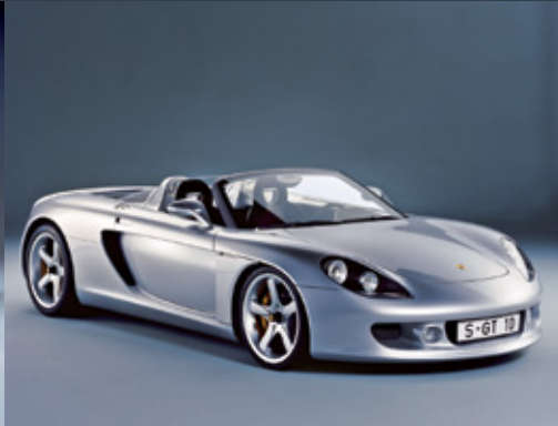
2003 The Carrera GT made its debut with an exceptional power-to-weight ratio of 443.4 hp per tonne (weight-to-power ratio of 2.25 kg/hp). The monocoque was made of carbon-fibre reinforced plastic (CRP).
