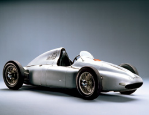
1947 The Cisitalia racing car developed under Ferry Porsche already featured a particularly lightweight magnesium body.
