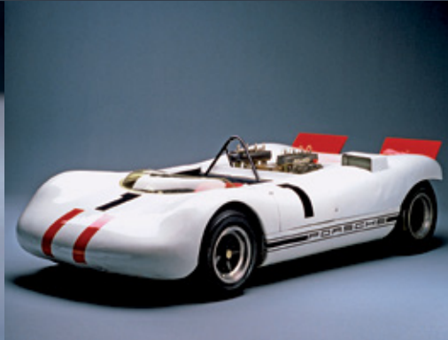
1968 The 909 Bergspyder weighed in at approx. 375 kilogrammes thanks to the use of beryllium, titanium, magnesium and aluminium.
