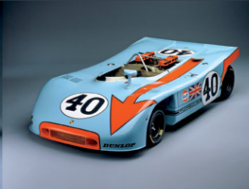
1970 With its particularly light tubular frame made of glass-fibre reinforced plastic (GRP), the Porsche 908/03 featured an exemplary lightweight construction.
