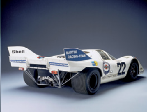
1971 The 917 KH short tail racing car had a magnesium frame. Gijs van Lennep and Helmut Marko set a track record at the 24 Hours of Le Mans.
