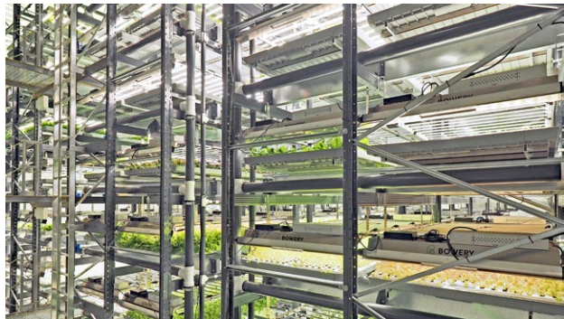
FIGURE 14 BOWERY FARMS IMPLEMENTING A HORIZONTAL STATIONARY DWC VERTICAL FARMING METHOD
