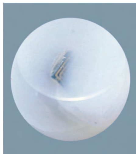
Figure 5: A composite shell bead that has been sliced and polished to show a small RFID chip (3 mm long) embedded within it. The information on such a chip can be accessed using an RFID reader. Photo by H. A. Hänni.
