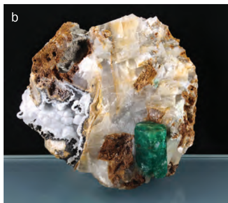
Figure 9: (a) Deep within the tunnels at Peñas Blancas, a white calcite vein (approximately 9 cm wide) shows typical orangy brown iron staining. (b) This mineral specimen from Peñas Blancas features a 2.5-cm-long emerald crystal embedded in the typical matrix of iron-stained calcite with a later secondary coating of botryoidal white calcite. Photos by E. Boehm.
