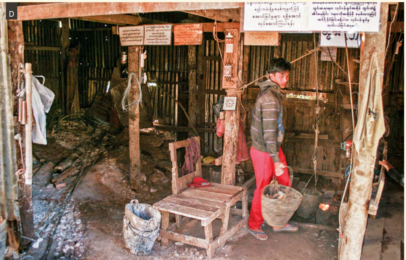
(A) The mined material is washed in a large triple jig. (B) A relatively new excavator works a portion of the open pit. (C) Workers sort through material that has been recrushed and washed. (D) Material is hoisted from a small mine shaft. Explosive charges hang from the pole on the far left.
