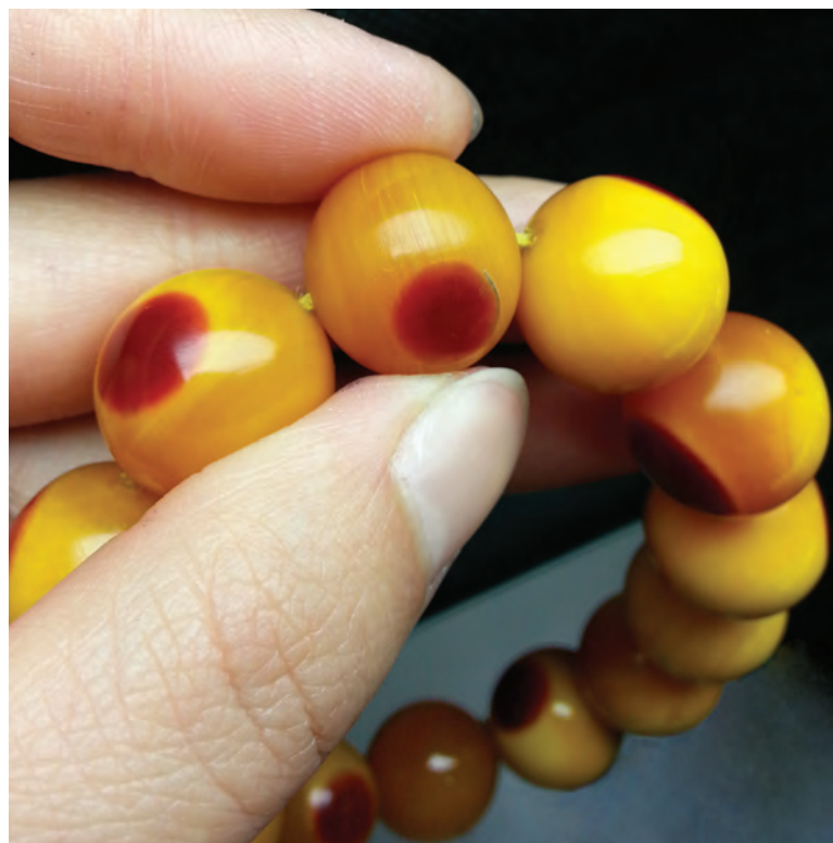
Figure 1: Hornbill ivory is a rare gem material that has been fashioned into a variety of decorative objects and jewellery, such as this beaded bracelet (average 17 mm in diameter; sample no. 8 in Table I). Three of the beads turned out to be composites made of genuine hornbill ivory and red resin. Photo by Jie Liang.
