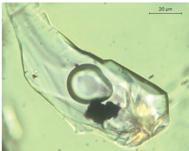
Figure 6: This multiphase C-H-S fluid inclusion in an unheated Merelani tanzanite comprises H_2S -rich liquid and vapour (distorted bubble), as well as solid graphite (opaque mass). Photomicrograph by D. Taylor.
