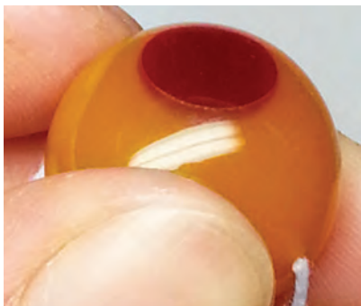
Figure 6: This imitation hornbill ivory bead from a bracelet (sample no. 7; 16 mm in diameter), shows a sharp and regular colour boundary. It appears that the red portion was set into the yellow area and then the sample was fashioned into a bead. Photo by Jie Liang.
