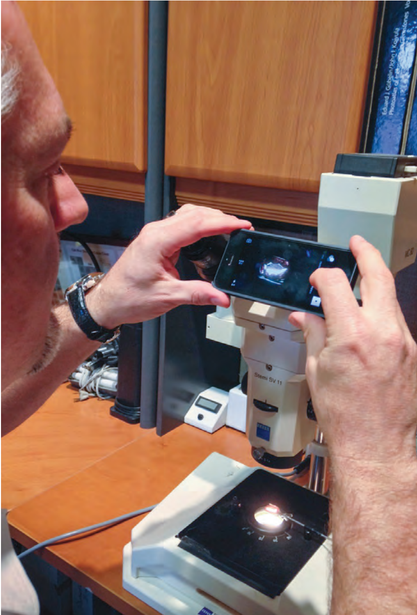
Figure 3: The author demonstrates the technique for taking photomicrographs using a smartphone camera. Here the lens of the camera is positioned over the right ocular, and the left hand is resting on the left ocular for stability. The camera lens is held approximately 1 cm above the ocular. Photo by Carley Boehm.
