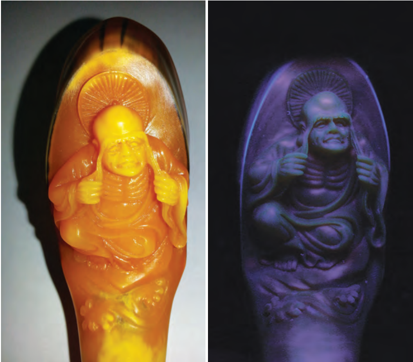
Figure 9: Sample no. 4 is shown here in incandescent light (left; photo by Jie Liang) and under long-wave UV radiation (right; photo by Haibo Li). The main orangey yellow portion is inert, while the thin red edge of the sample displays moderate bluish fluorescence.
