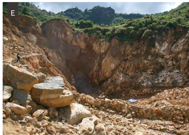
(A) A peridot miner rests next to buckets containing powdered rock and rolls of explosives. (B) This pendant containing a large faceted peridot gemstone was seen in Mogok. (C) Miners excavate gem-bearing soil at Pyant-Gyi, a source of high-quality red spinel. (D) Women search for gems at Pyant-Gyi. (E) Residual deposits are mined from weathered karst in this open pit at Htin-Shu-Myaing. Photos by M. Lorenzoni (A–D) and F. Pezzotta (E).
