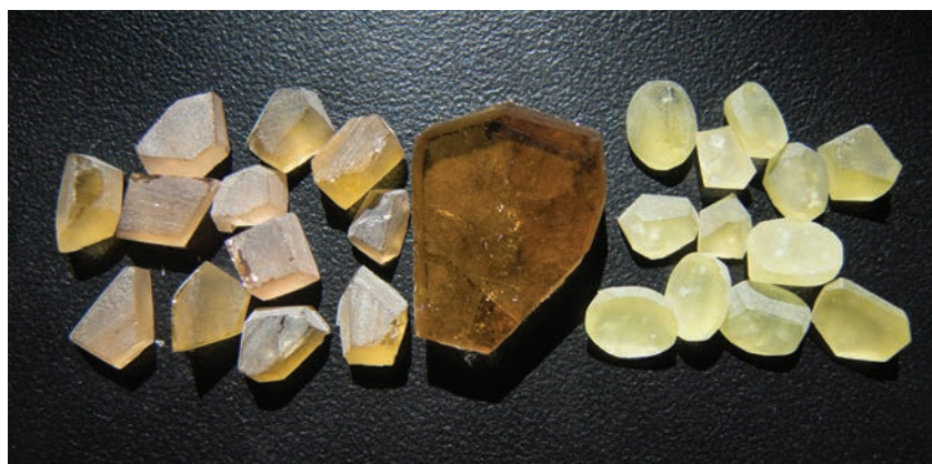
Figure 13: These tourmaline pre-forms were cut from material that was mined from a primary deposit at Mavuco, Mozambique. The brownish yellow colour shown by the stones on the left and centre changed to light yellow with heat treatment, as seen in the pieces on the right. No copper was detected in the samples, which have a total weight of 63.45 carats; the largest piece (which has been partially polished) weighs 21.12 ct and the smallest is 0.86 ct. Gift of Mozambique Gems; photo by B. M. Laurs.
