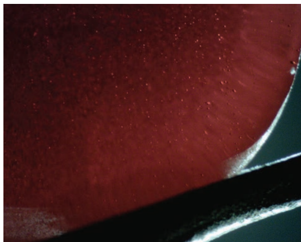
Figure 19: Numerous rounded gas bubbles are present in the star CZ, which appears brownish red under strong illumination. Photomicrograph by B. Deljanin; magnified 30×.
