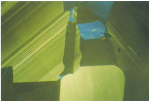
Fig. 5. Typical growth sectors in the experimental synthetic diamonds with characteristic double bell-form of 111 sectors intensely banded, and bright greenish-yellow 001 sector. Intercalated blue and dark green sectors resembling higher indexed faces. Cond. excit.: 12 kV, 0.9 mA. 28x (24 x 36mm).
