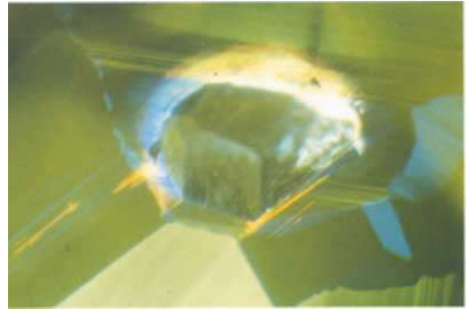
Fig. 4. The same large crystal inclusion as Fig. 3 during electron bombardment. Note greenish-yellow CL colour, stress-induced cloud around the crystal and fine orange-red needles barely visible in transmitted light. Blue CL colour indicates lower N-concentration, irregularly distributed. 43x (24 x 36mm).
