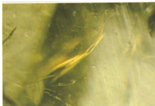
Fig. 5(a) and (b). Colour flashes in feathers seen in a resin treated emerald (Photographs R. Kammerling).
