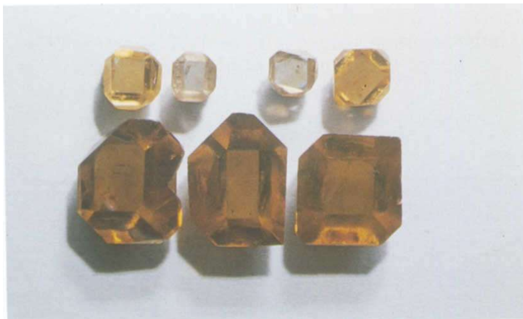
Fig. 1. Set of 7 experimental synthetic diamonds made by De Beers. Top row, left to right: DMY-4 (0.97 ct), DMY-6 (0.40 ct), DMY-10 (0.44 ct) and DMY-5 (1.03 ct). Bottom row, left to right: DMY-1 (5.24 ct), DMY-2 (4.57 ct) and DMY-3 (4.10 ct). Note cubo-octahedral habit and natural colours. 2.6x, incandescent light.
