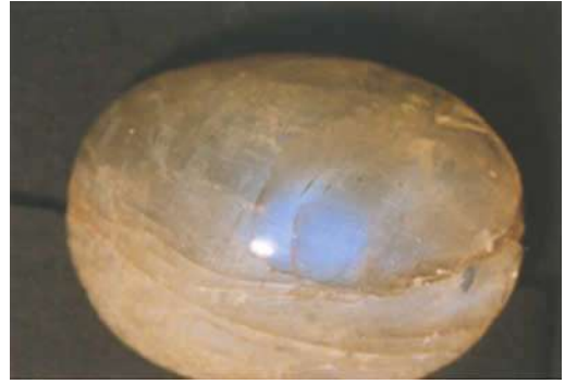
Fig. 8. Blue moonstone in a crystal blue quality (size of the sample: 58 \times 45\text{mm} ). The clear transparent and colourless area of the moonstone is limited by a tight net of cleavage and cracks. The size of cut moonstone from this sample could only be up to 7mm. This pegmatite occurs near the plate tectonic border of the island. This geological fact is the reason why cut moonstones from Metiyagoda mostly occur in small flat pieces.
