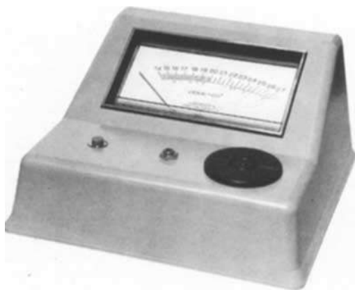
Fig. 1. The Sarasota Instruments 'Gemeter '75' – one of the first reflectance meters.
