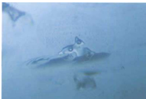
Fig. 6. Heat altered inclusion in sapphire.
