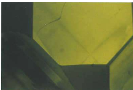
Fig. 14. Same stone (DMY-7) as in Fig. 11 showing dark Maltese cross on greenish-yellow luminescing octagonal growth sector at higher magnification of 28x (24 x 36mm). Same cond. excit.
