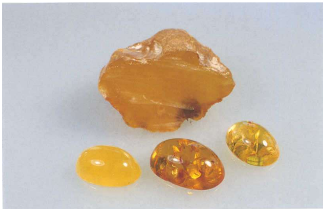
Fig. 4. Rough amber and three cabochons cut from the same material. Bottom, from left to right: before heat treatment, after heat treatment, and after heat treatment and repolishing.
