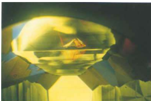
Fig. 13. Same stone (DMY-7) as in Fig. 11 with one 111 growth sector containing large inclusion surrounded by orange-red needles of unknown composition. Higher indexed faces luminescing steel blue. Cond. excit.: 11 kV, 0.9 mA. 10x (24 x 36mm).
