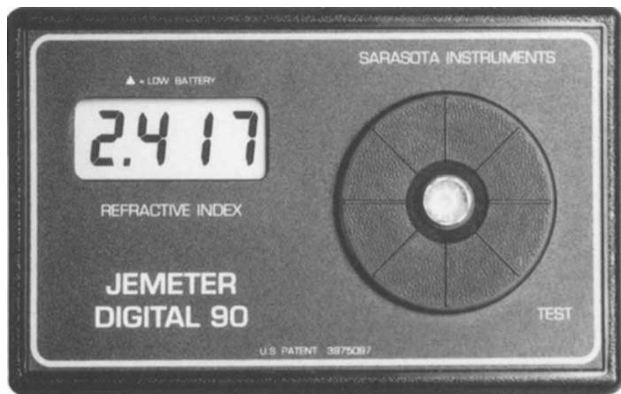
Fig. 2. The Sarasota Instruments 'Jemeter Digital 90' reflectance instrument measures gemstone RIs to three decimal places over the range 1.450 to 2.999. Fitted with a polarizing filter, it can also measure double refraction down to around 0.01.
