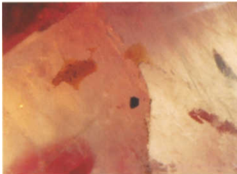
Figure 9: Mineral assemblage with ruby and a black picotite grain in a matrix of colourless anorthite. Photo by K. Schmetzer, magnified 80 x.
