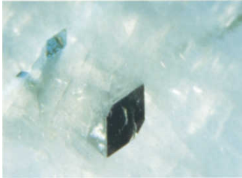
Figure 8: Cross section of a prismatic pargasite crystal consisting of four {110} and two smaller {010} prism faces. Photo by K. Schmetzer, magnified 60 x.
