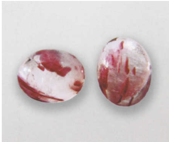
Figure 1: Ruby crystals in a matrix of colourless anorthite. Size of the sample on the left: 10.5 × 8.3 mm; photo by M. Glas.
