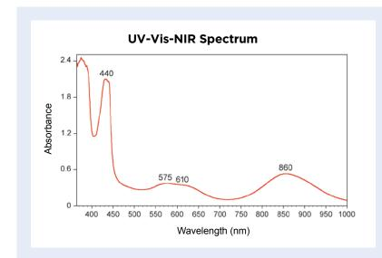
**Figure 5:** The UV-Vis-NIR spectrum of the andradite displays features related to Fe<sup>3+</sup>: a distinct peak at 440 nm, a weak broad doublet at 575 and 610 nm, and a stronger absorption at 860 nm.
