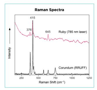
**Figure 12:** A representative Raman spectrum of one of the rubies is compared to a corundum reference spectrum and shows sufficient similarity to confirm its identity.
