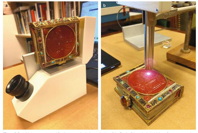
Figure 6: Portable instruments used for the gemmological examination of the Book of Hours included (a) a refractometer and (b) a Raman spectrometer with a 785 nm red laser. Photos by G. Panczer.
