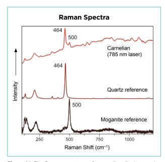
**Figure 14:** The Raman spectrum of a carnelian displays peaks corresponding to quartz (464 cm<sup>-1</sup>) and moganite (500 cm<sup>-1</sup>), as compared here to reference spectra from the RRUFF database and Schmidt *et al.* (2013), respectively.
