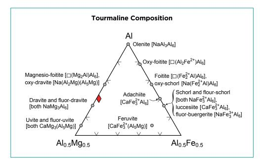
**Figure 4:** A triangular diagram with total Al-Mg-Fe (apfu) shows the chemical composition of the blue Elahera dravite (red diamond symbol). Ideal chemical compositions of Li-free, Al-Mg-Fe tourmaline end members (cf. Bosi 2018) are shown by grey circles. Only the XY<sub>3</sub>Z<sub>6</sub> cations in the formulae are given.
