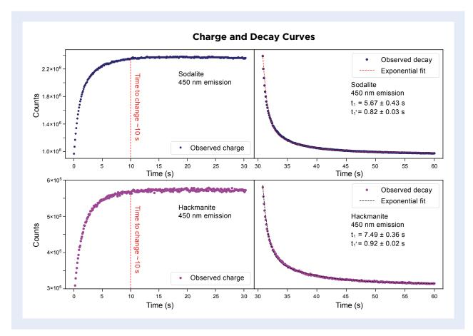
**Figure 19:** Charge (left) and decay (right) curves are shown for the colourless sodalite and the hackmanite. The charge curve indicates that the intensity of the blue luminescence reaches a maximum after about 10 s. The fit of the decay curve includes a combination of two exponential functions, corresponding to decay times of about 1 and 6 s.
