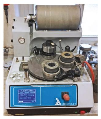
**Figure 4:** A Logitech automated lapping and polishing machine was used to grind the samples for 30 minutes for this study. At the top, a rotating barrel contains the abrasive slurry. On the steel lap are two oscillating sample discs, weighted down with 4 kg of lead. At the back of the lap, a diamond-charged dressing tool keeps the lap wheel flat. Resting on the front-left side of the machine is a glass disc affixed with six magnesite samples. Photo © H. A. Hänni.
