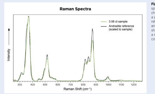
Figure 4: The Raman spectrum of the colourchange garnet provides a good match to the reference spectrum for andradite and does not show the presence of a significant grossular component.
