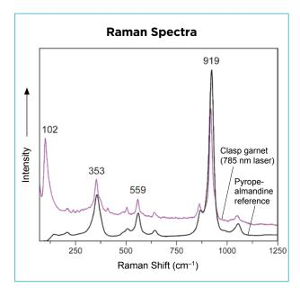
**Figure 15:** The Raman spectrum of the clasp stone provides a good match to that of a pyrope-almandine reference spectrum.
