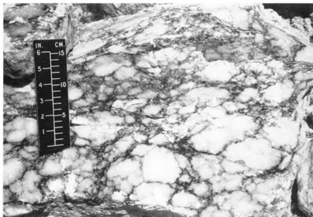
FIGURE 10—Characteristic nodular gypsum, Todilto Gypsum Member; San Felipe Quarry, Tonque Arroyo, Sandoval County, New Mexico (SW¼ sec. 1, T13N, R5E).
