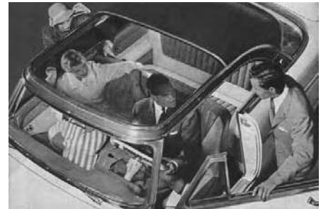
Monterey 2-Door Sun Valley Hardtop roof detail
