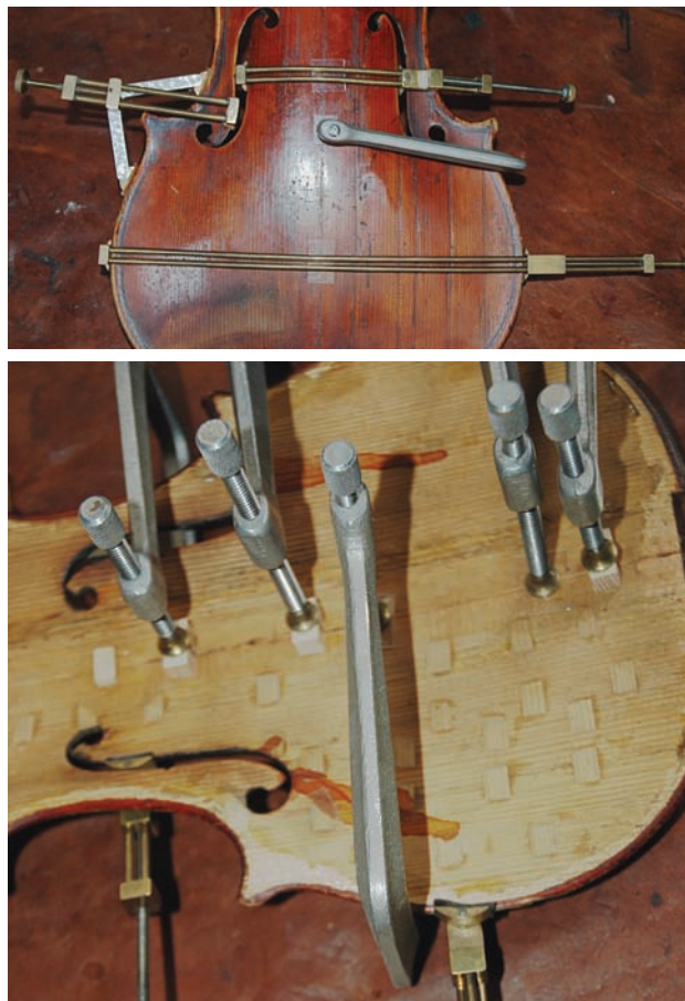
Figure 3 Stretcher clamps (top) and aluminum double-swivel clamps (bottom) in use. Photos: Jonathan Woolston.
