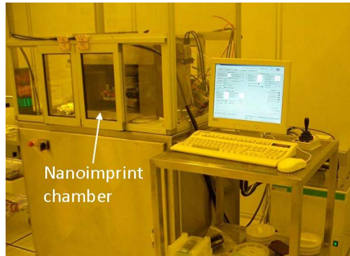
Figure 3.8. NIL available at the clean room of the IMB-CNM institute.
