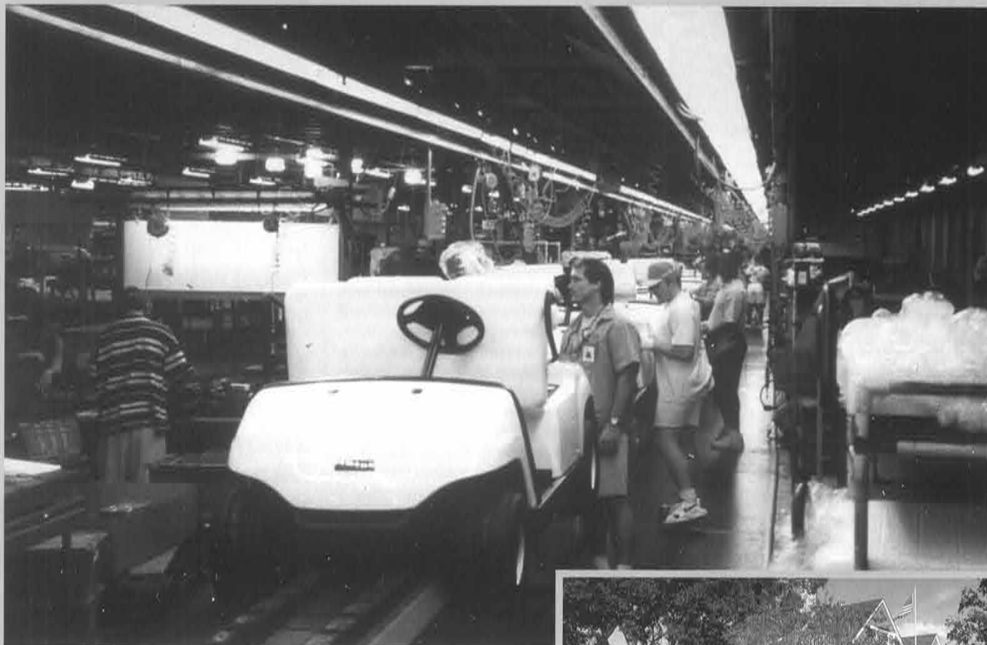
Golf Car assembly line in the YMMC factory
