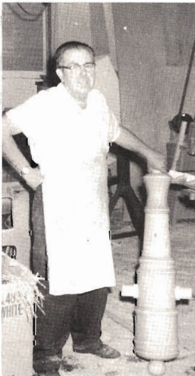
Gun pattern was turned from two planks to separate when placed in two-piece mould. Pouring gun (above) took 400 pounds of metal. Bore was made from steel tube laid in mould.
