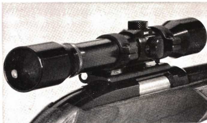
Scope in swing-out mount fits gun for occasional shots at long range, makes iron sights available for close-in work.
