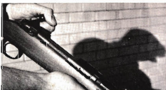
Author checks first factory-made U.S. bolt rifle built for left-handers. Collar forward of action locks barrel into place. Combination sear and bolt stop (at left) are on right of receiver like regular M110. Running shells through bolt gun without taking it from shoulder was new experience for GUNS' Tech Editor Bill Edwards, who is left handed.
