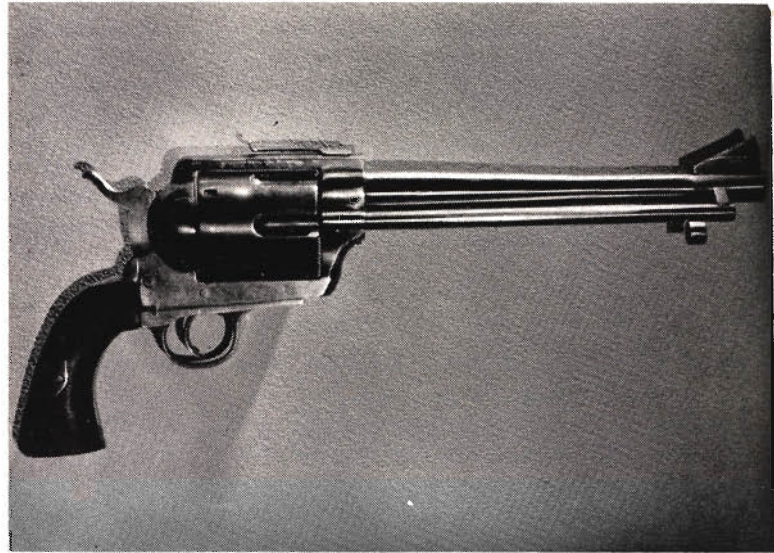
Shown in recoil at left, revolver above was made by R. G. Wilson and Wm. Howe, weighs 6 lbs. 2 ozs., pitches a 405 grain bullet at an estimated velocity of 1600 ft. per sec.
