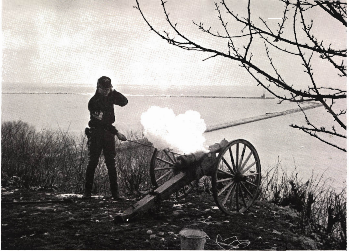
Cannoneer Carpenter touches off home-made two-pounder in great guns shooting match held just after finish of article telling how he made cannon. Projectile is concrete-filled tin can.
