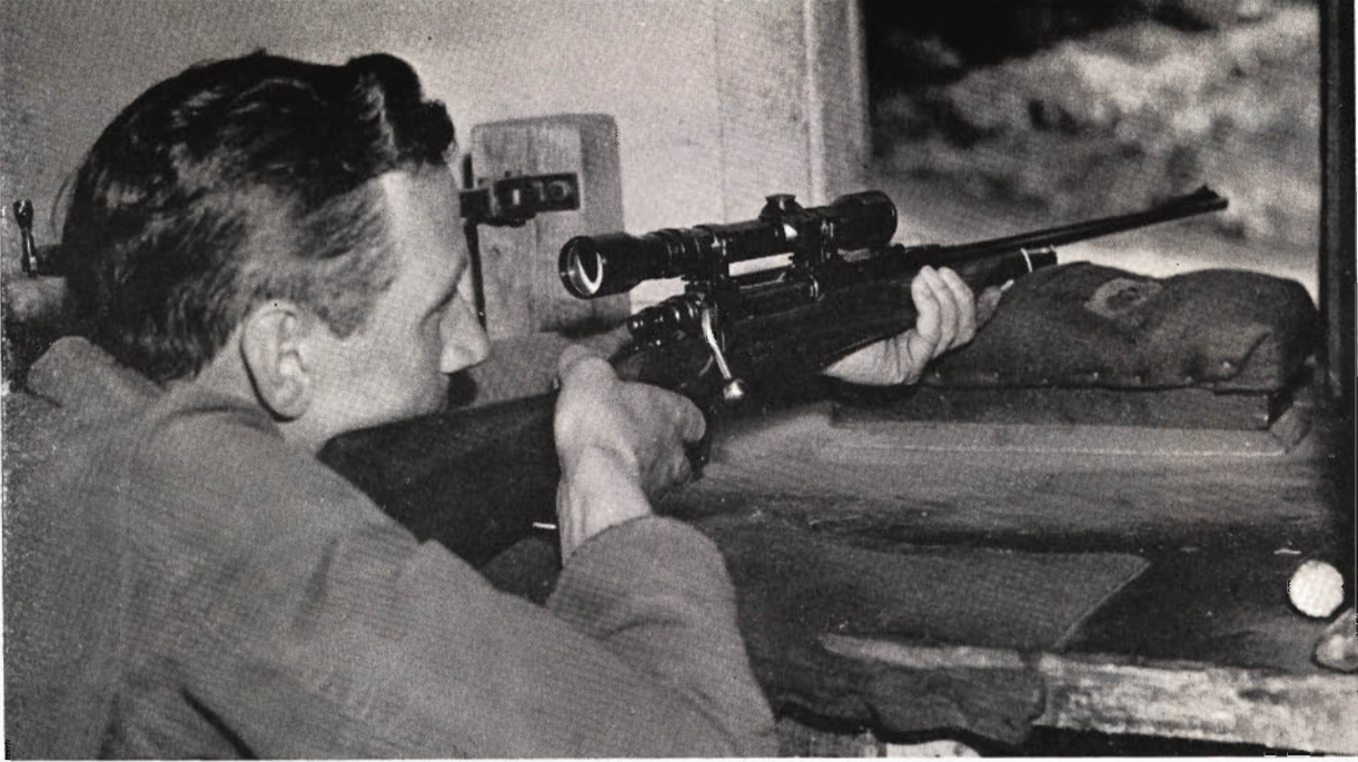
Sighting-in rifle over 100 meters, inspector checks HVA rifle for close groups using Norma ammunition before OK.
