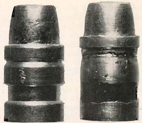
Bullet at right, pulled with inertia bullet puller, shows deformation due to excessive crimping of case mouth.
