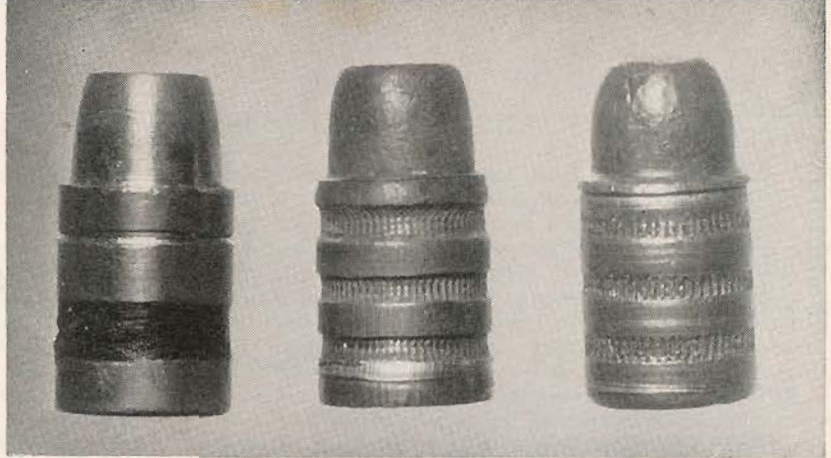
Above: A bullet cast in Hensley & Gibbs No. 51 mould (left) has more efficient shape than factory .357 slugs. Left: These perfect .30 caliber castings are shown before and after lubricating and sizing.
