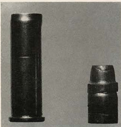
Left: A bullet pulled from reload shows bad fold in nose and deformed groove due to excessive crimp of non-uniform case wall. Right: Cast shank in bullet base or hollow point nose, used to lap rusted mould.
