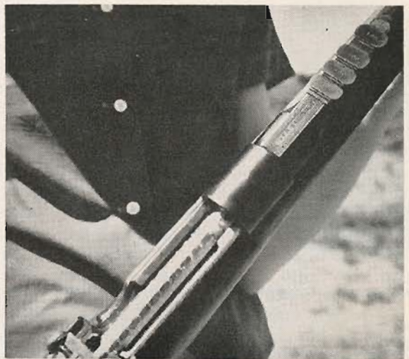
Folding leaf express sights, common on double and bolt action German rifles, are seldom seen on British-made doubles used by white hunters.
