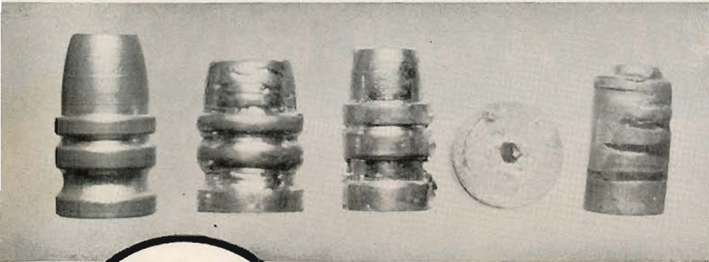
Left to right: A perfect casting; cast with wrinkles (cold alloy); fins (by sprung blocks); hole in base (sprue not solidified); out of line sizer.
