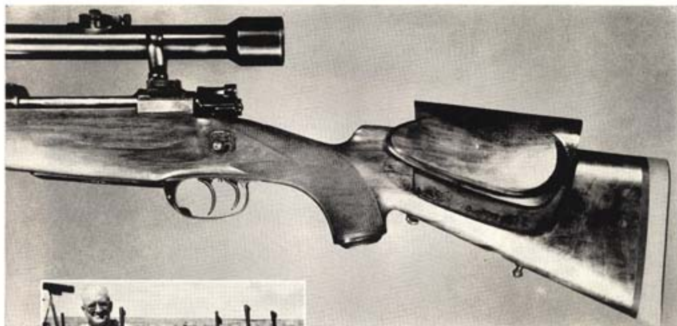
Goering's 9.3 x 70 Schwy-Mauser shows stock evolution, shapes to reduce kick. Cheek piece slants away from cheek bone; long pistol grip curve avoids finger bruise.
