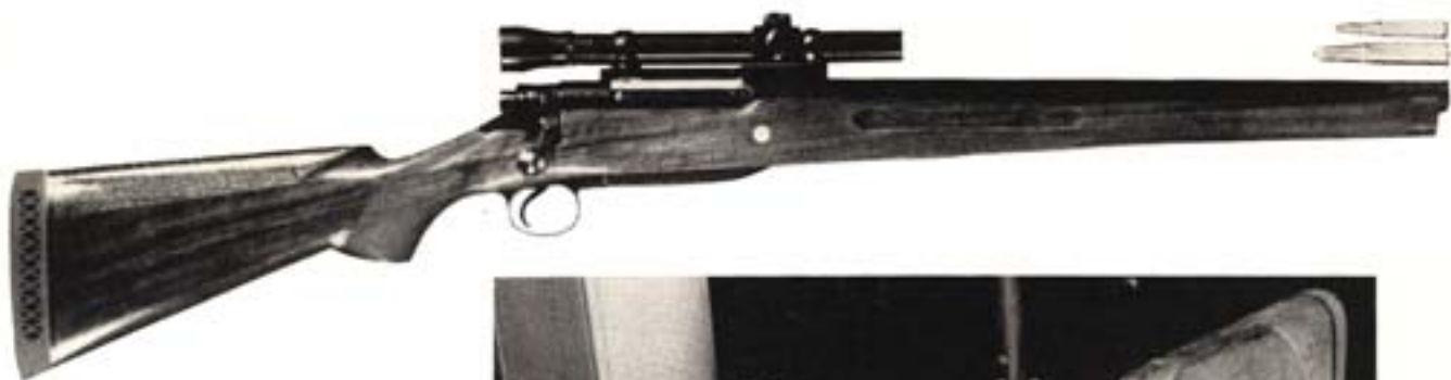
Zero-pitch stock with butt pad at right angle to line of bore aids in reducing kick but height of thrust—axis of bore—above shoulder still makes Buehler's .505 Gibbs a bruiser. At right, Holland double .600 made for late King Faisal II of Iraq shows straight stock necessary to hold the jolt.
