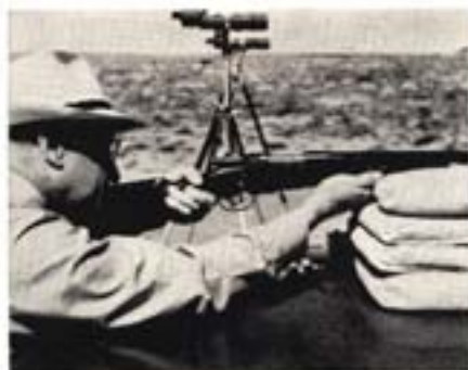
Misplaced trigger puts 2nd finger against guard where kick can hurt.
