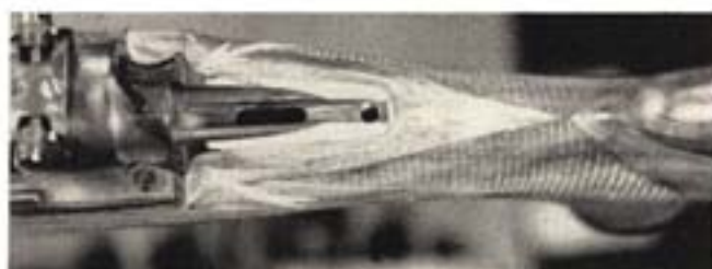
To avoid splitting small of stock, action should not bear at two rear inside radii and at tang tip. Even with recoil lug solid, stock will "give" over magazine.
