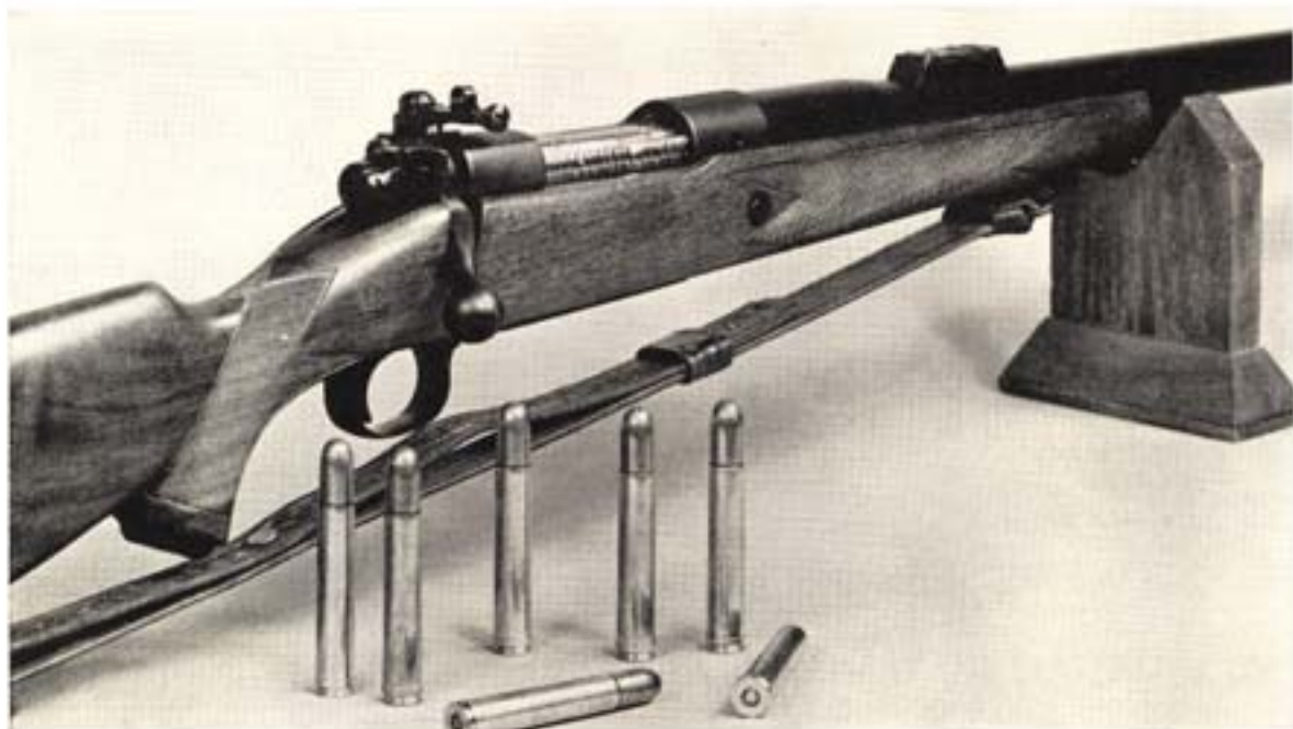
Although big Winchester "African" in .458 Magnum is precision-inletted to gauge at factory, bolt with square section steel bar is needed at recoil lug recess to avoid splitting the stock. Metal must not wedge wood apart in inletting.
