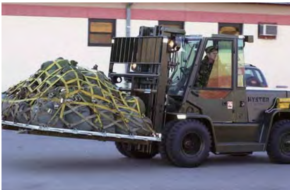
A typical 463L pallet, here shown being transported by a 15,000-pound forklift
