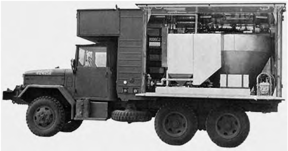
Reverse-osmosis water purification unit; below , A typical erdlator
