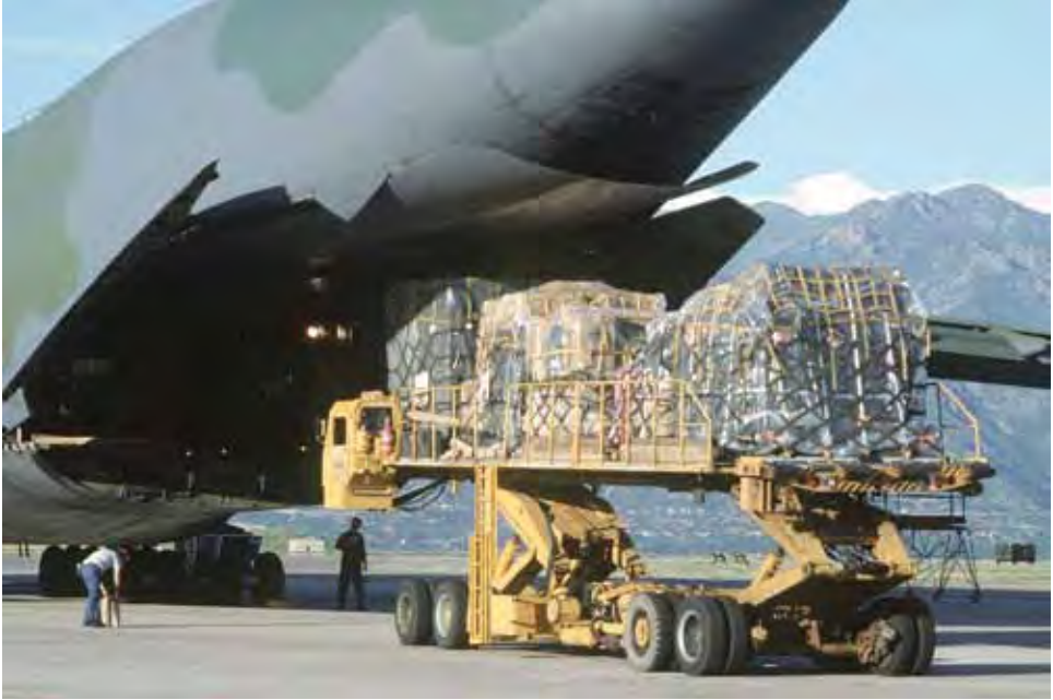
A typical K-loader, here shown loading equipment aboard a C-5A during an exercise
