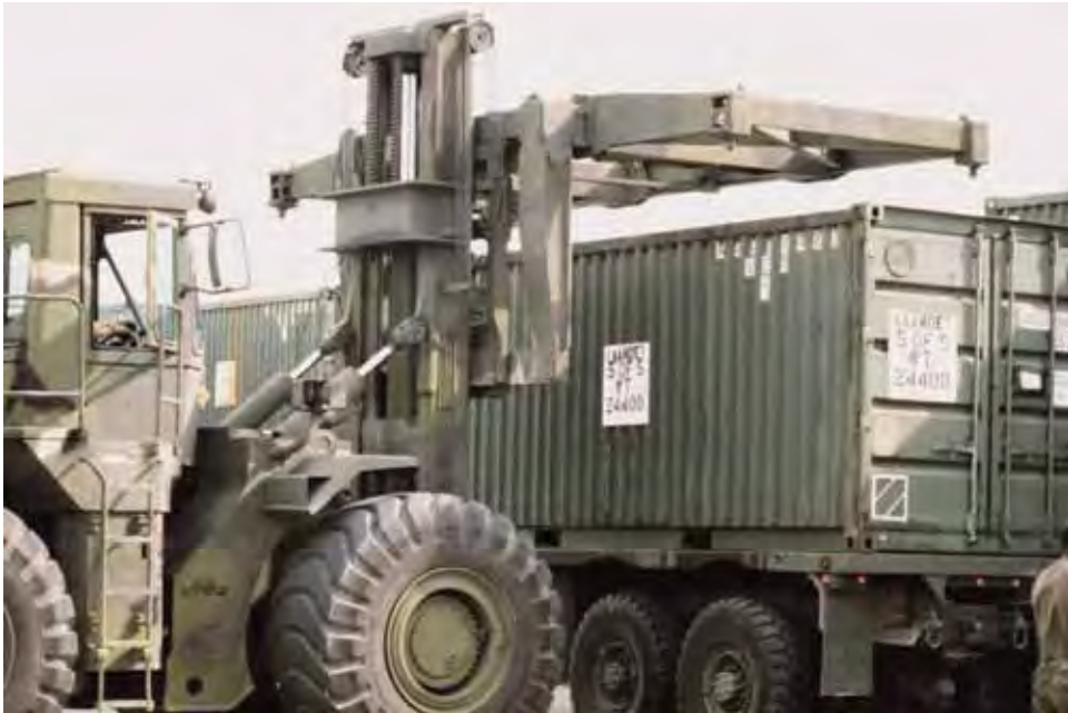
A 10,000-pound forklift backs away after placing a CONEX on a trailer.
