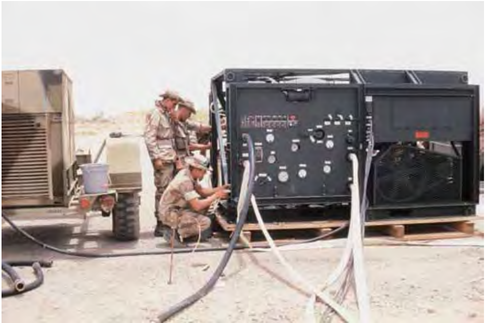
Reverse-osmosis water purification unit; below , A typical erdlator
