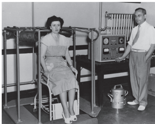
FIG. 1. Dr. Saul Hertz using a multiscintillation counter that he designed to analyze the distribution of radioactive iodine in a volunteer. With permission from the Dr. Saul Hertz Archives.
