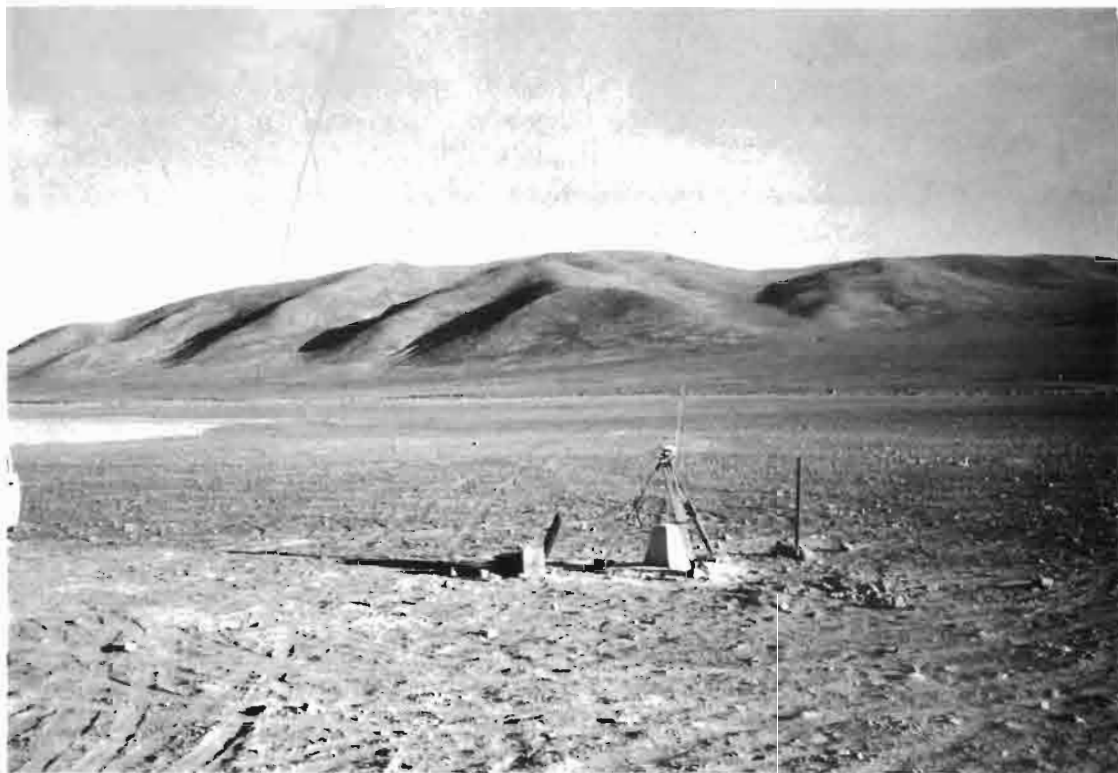
Fig. 3.2.1.- GPS benches of the North Chile network set up in 1992: these were monitored in the weeks following the 1995 Antofagasta earthquake. Above, at Chacaya (S of Hornitos) ; below: a station SE of Antofagasta, on the road to La Escondida (Photos L.O.).
