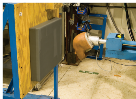
A head-strike cannon is used to test the HOPS cushion system
