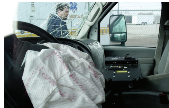
More than 30 years of impact testing did more than create a baseline for HOPS development. Horton testing validated the structural integrity of the body, as well as the patient area. This validation is unmatched by any other ambulance manufacturer.
