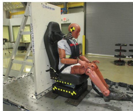
Like any collision protection system, HOPS is effective only when occupants are wearing seat belts. CPR, head and aft bench seat belts have detachable four point belts to enhance mobility.
