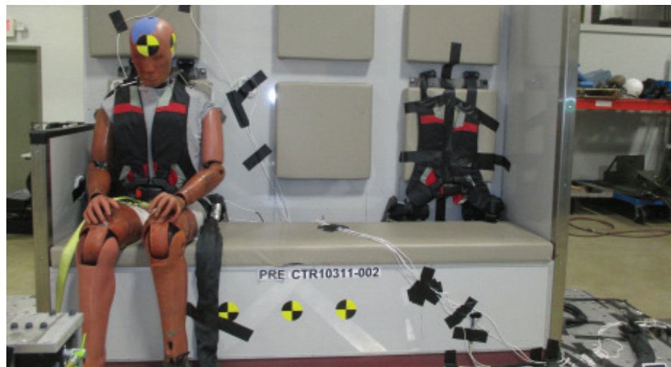
The Horton Occupant Protection System (HOPS) is fully tested and combines advanced restraints, multi-density head protection, tubular airbags and head curtain airbags to protect attendants in side impact rollover crashes.
