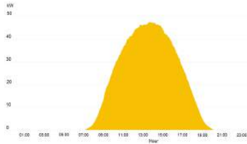
Fig. 3. Hourly distribution of photovoltaic production for the day 27/05/2022.
