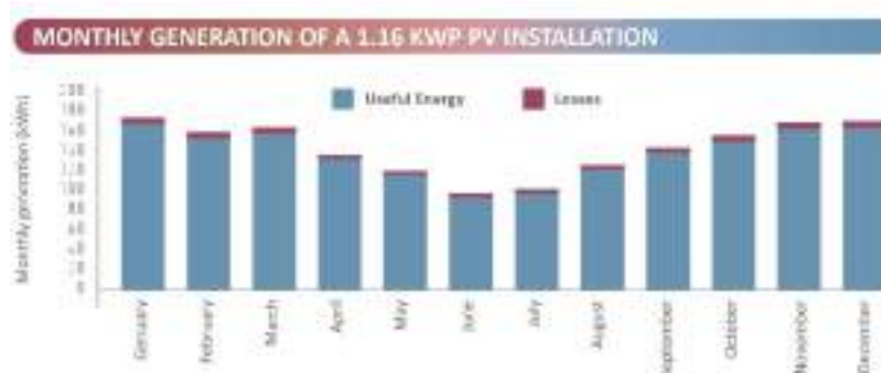
Fig. 5. Monthly simulation for a 1.16kWp PV system in Buenos Aires (1650 kWh/year (±10)).
