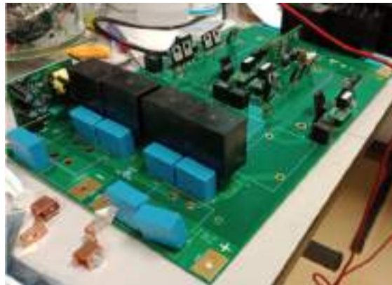
Fig. 5. DC/DC photovoltaic converter in development.
