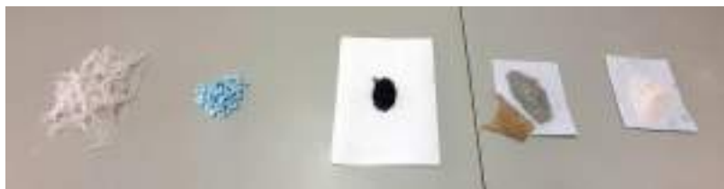
Fig. 2. Different additives selected to be used in the mortar mix. From left to right: polyester fibres, polystyrene, graphite, crystallised gypsum and gypsum powder.
