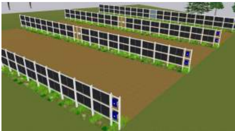
Fig. 1: Vertical bifacial facility for agrivoltaics.
