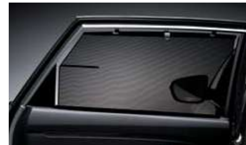
2 nd row sun blind The manually retractable sunshades for the 2 nd row windows provide protection from harsh sun glare and help to keep the cabin cool.
