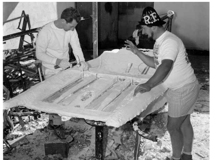
Roth's plaster and fiberglass building method can be seen here as he (right) oversees work on 'the Wishbone.' Photo by Bud Lang/The Enthusiast Network/Getty Images)
