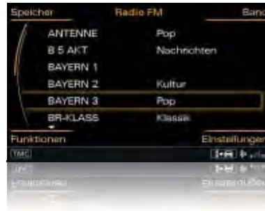
Radio: The integrated radio receiver is set up for VHF, LW and MW and optionally transmits digital radio with a continually updated station list.
