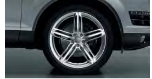
Audi exclusive cast aluminium wheels in 5-segment-spoke design 2 size 10 J x 21 with 295/35 R 21 1 tyres, including wheel arch trims 3 . From quattro GmbH
