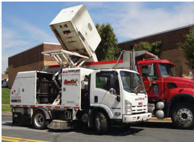
The Starfire S-4 mechanical broom street sweeper by Stewart-Amos Sweeper Co. is mounted on a highly maneuverable, fuel efficient, non-CDL chassis.
