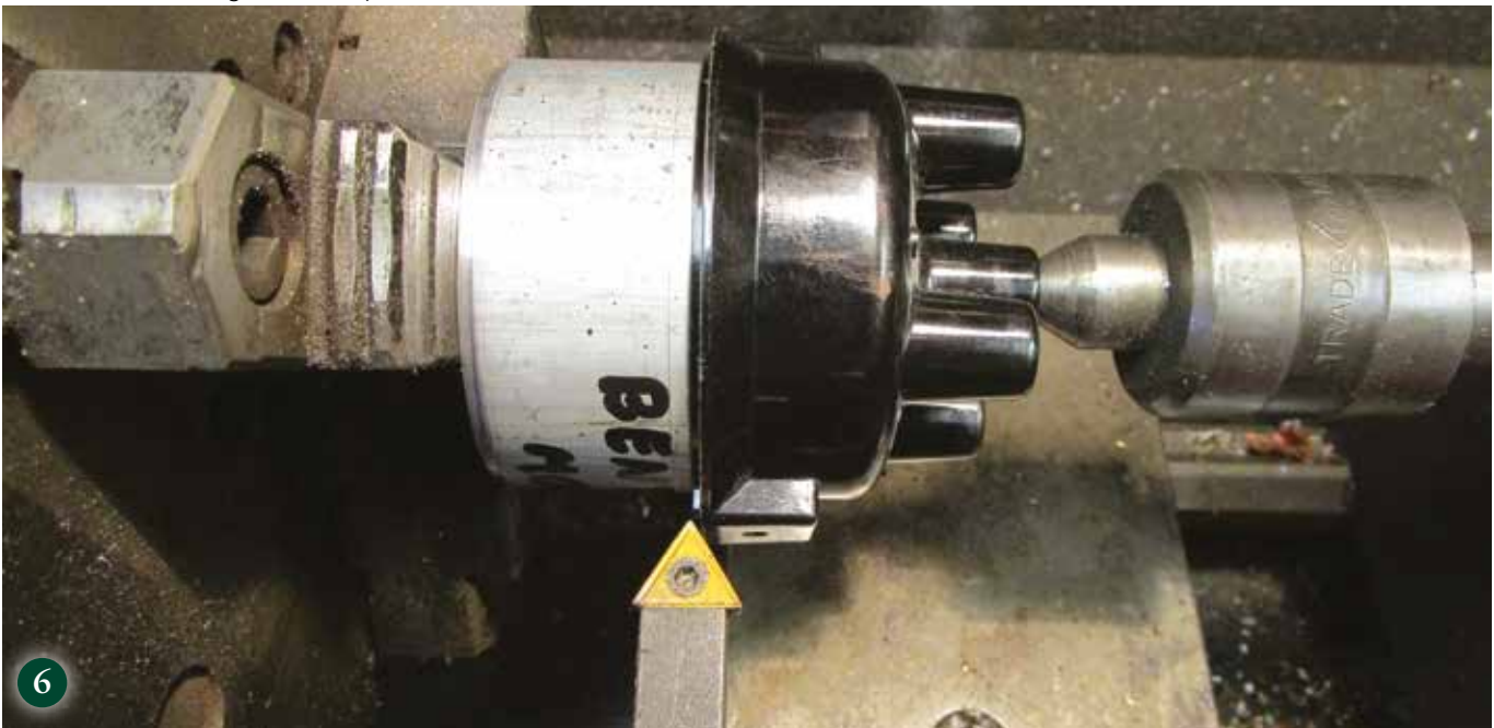
6 The DR-405 cap mounted on the lathe ready for turning
