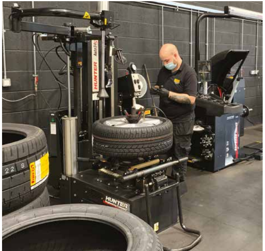
The state-of-the-art Pirelli Performance Centre boasts a special tyre removal machine, designed to ensure that no metal parts scrape or scratch the alloy wheel
