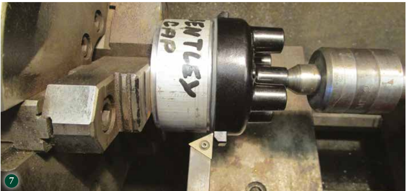
7 The fully machined cap, with the bosses (used to hold the spring clips on the magneto) being the correct height for a tight fit
