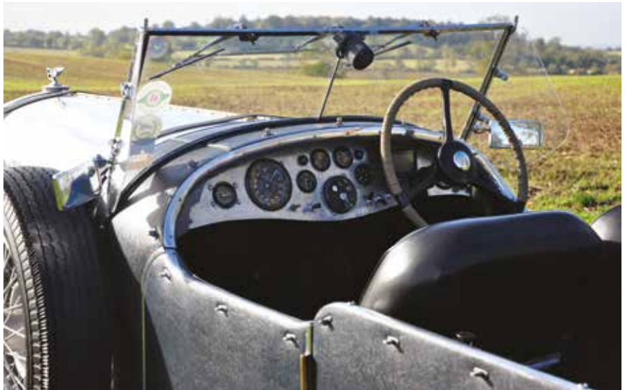
Full windscreen protection ensures the R Type is a true touring car while a tachometer complements the car's instruments
