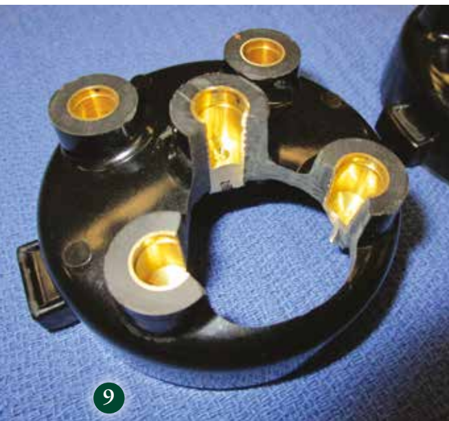
An exposed machined cap showing the central contact and contacts for the spark plug wires
