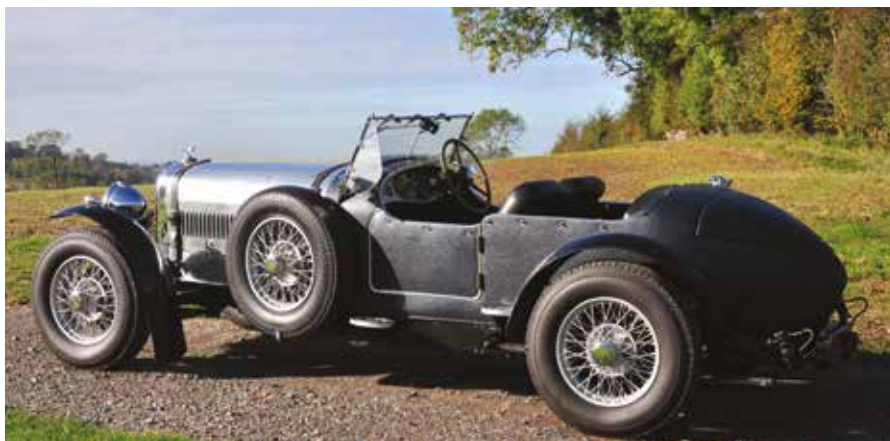
The shortened R Type chassis has tailor-made doors, full weather equipment and a boot
