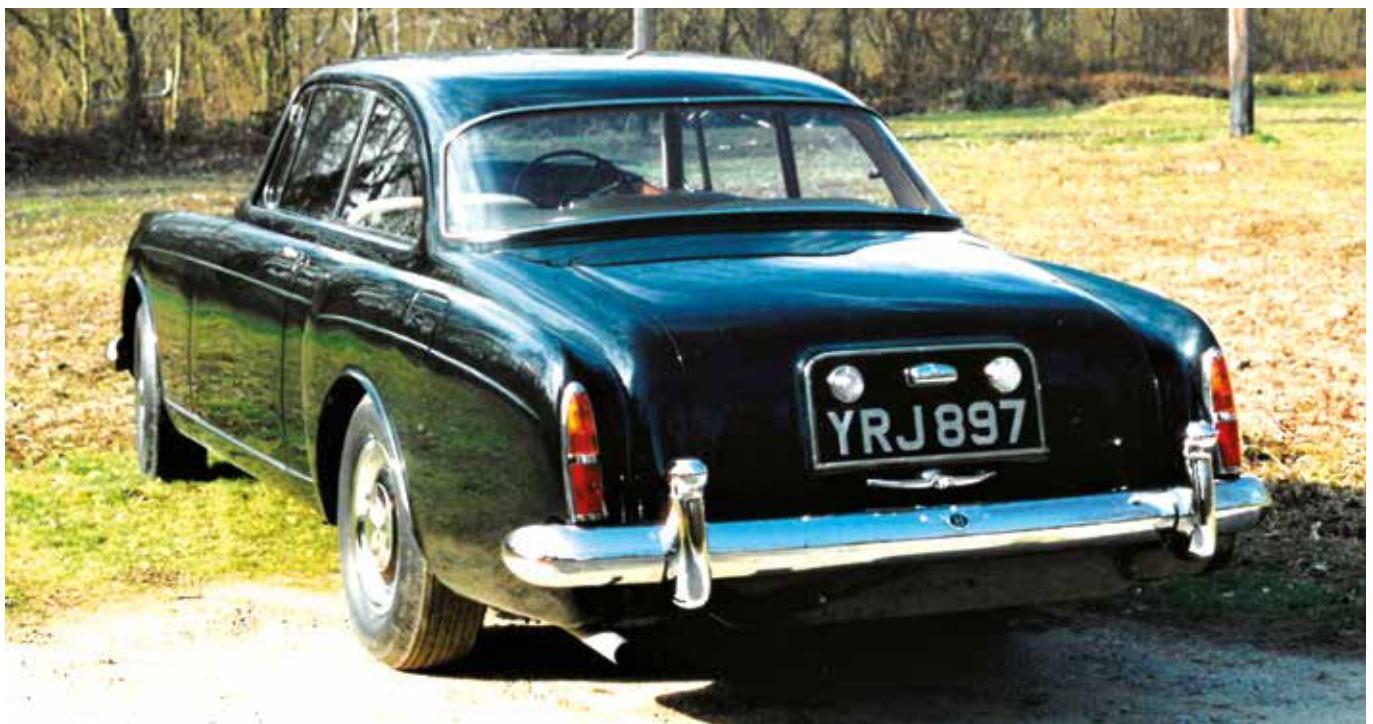
The S2 two-door coupé by HJ Mulliner was a development of the fastback, featuring notchback styling to increase boot space and rear passenger headroom
