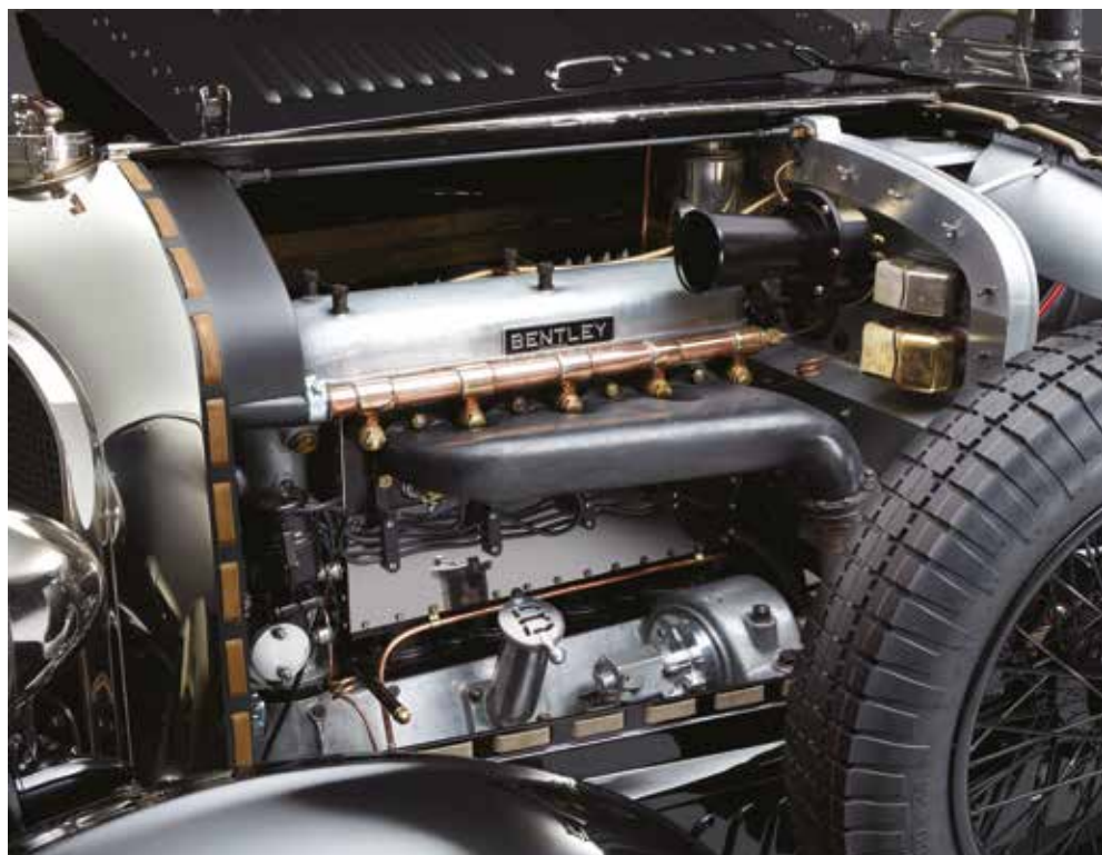
Modifications, including a large-bore 4 1/2 block, ensure a high level of performance
