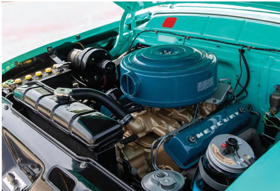
Under the hood is Mercury’s 312cid V-8 mated to an air-cooled Merc-o-Matic automatic transmission.
