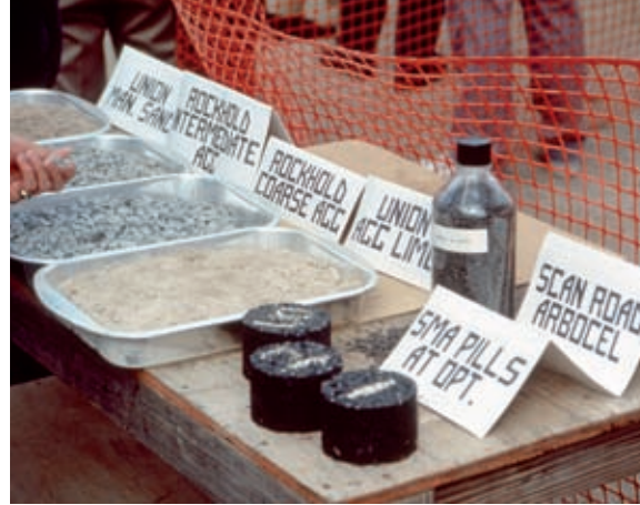
The European Asphalt Study Tour of 1990 introduced the U.S. paving industry to Stone Mastic Asphalt, displayed here.
