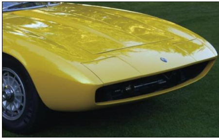
Figure 18. This very early Ghibli has several unique features including a ventless hood, no air inlet vents under the grille, and no marker lights. Courtesy of the Vintage Exotics Collection.
