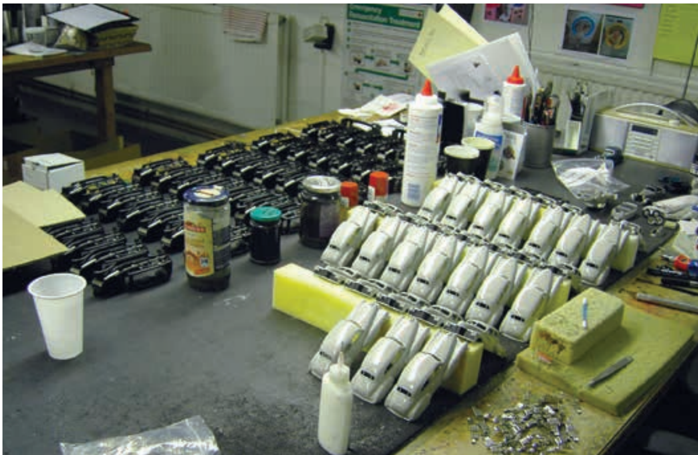
Another part of the assembly line with bodies propped up whilst the glue sets.
