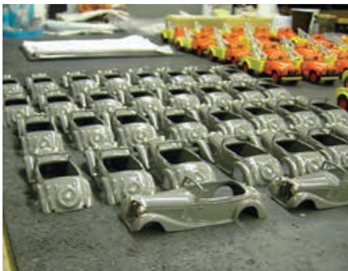
The first batch of Jensen Dropheads with brightwork attached to the painted bodyshells and awaiting bumpers, chassis and interiors.
