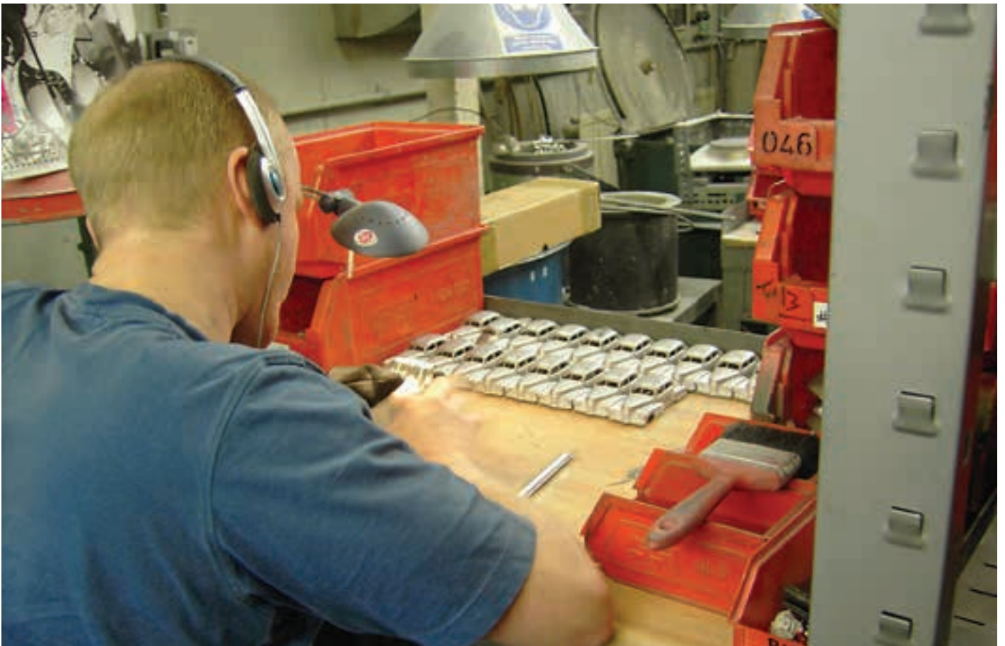
The casting room with a batch of bodies being cleaned up by hand.
