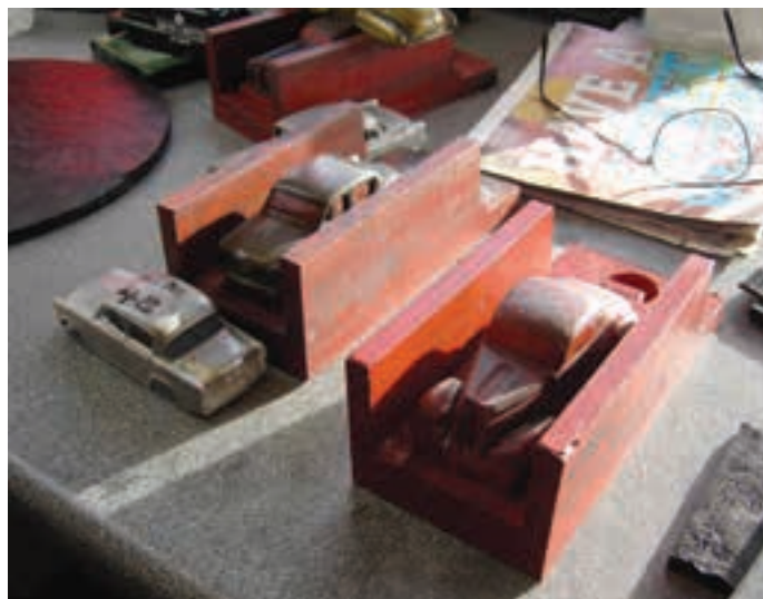
An early stage of mould making with the body of a Hillman Minx and rubber castings of other cars being worked on.
