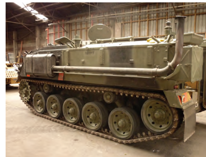
(Left, Above and Below) Mark Cameron's FV432 personnel carrier powered by a K-60 engine through this tiny hatch may bring a wry smile to many faces. This vehicle is completely amphibious and can operate in extreme climatic conditions. Other variations included mortar and Wombat anti-tank gun carriers and a REME (Royal Electrical and Mechanical Engineers) mobile workshop.
