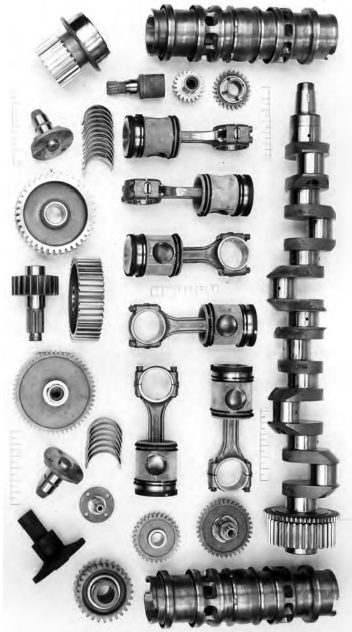
The major components of the K-60 engine. It is a relatively simple design with two crankshafts, six cylinders, 12 pistons and no valves.
