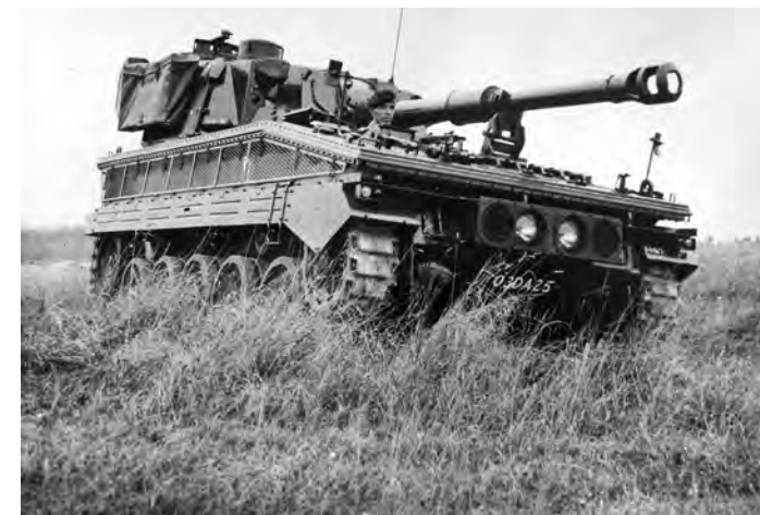
(Above) The FV430 Abbott self propelled 105mm gun which used a Rolls-Royce K-60 engine and an Allison six speed automatic gearbox which was manufactured by Rolls-Royce under licence. (Left) Truck – An all-terrain armoured truck powered by a K-60 engine.
