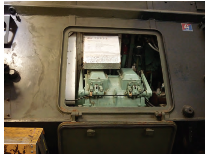
(Left, Above and Below) Mark Cameron's FV432 personnel carrier powered by a K-60 engine through this tiny hatch may bring a wry smile to many faces. This vehicle is completely amphibious and can operate in extreme climatic conditions. Other variations included mortar and Wombat anti-tank gun carriers and a REME (Royal Electrical and Mechanical Engineers) mobile workshop.
