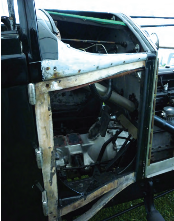
(Left and below) 1929 20 h.p., Sedan by Thrupp & Maberly on Chassis GEN51, at the Rolls-Royce Enthusiasts' Rally, Castle Rockingham in 2011, in original and un-restored condition, to display features of its construction, and its Chassis Build documents.
