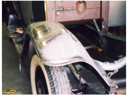
Left front fender was re-formed by an expert "metal bender" as the original was not salvageable. It cannot be told from new.
