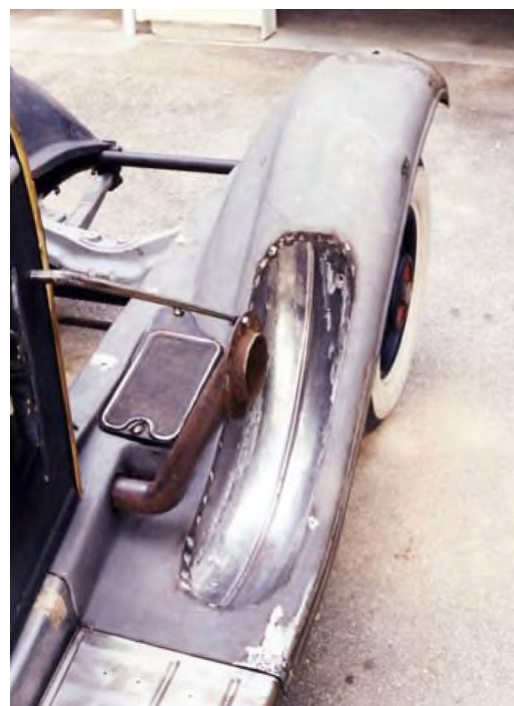
Above, the "new" right front fender with the wheel well. The original was too far gone to be repaired. A master metalsmith created a new one from sheet metal.
