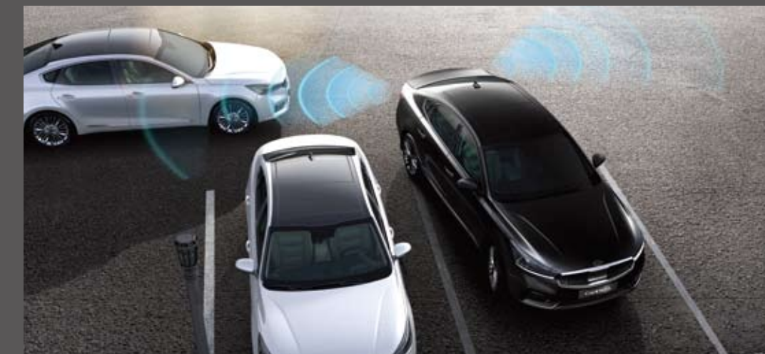
Rear Cross Traffic Alert (RCTA) When you back out of a parking spot or driveway, RCTA gives you a warning if it detects any cross traffic in the lane the vehicle is entering.
