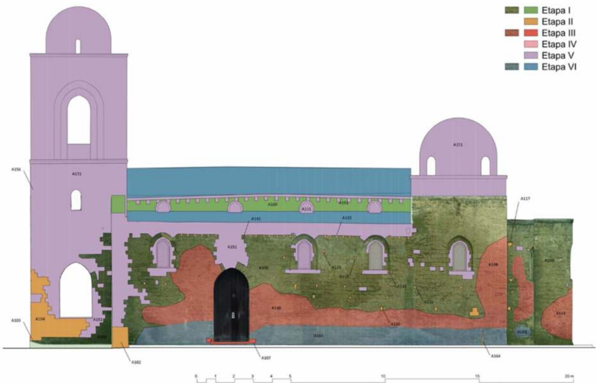
Figure 6 – Archaeological records of the south façade of San Giovanni
