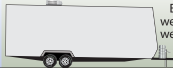
Excessive hitch weight
