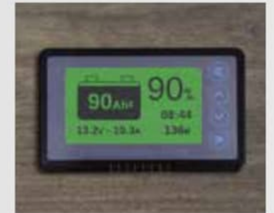
Upgraded battery monitor displays battery statistics like amp-hours consumed, state of charge, and voltage.
