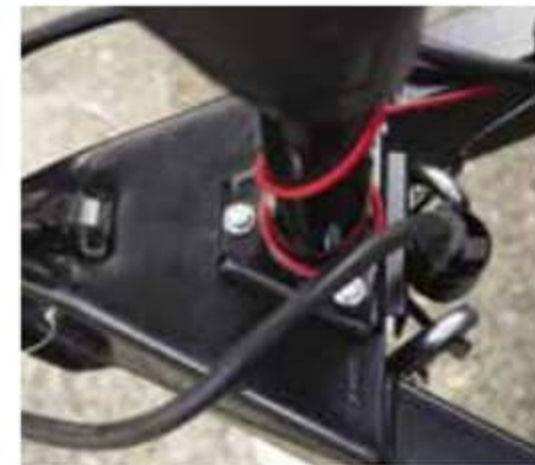
Electric cord and chain caddy. Keep these items off the ground.
