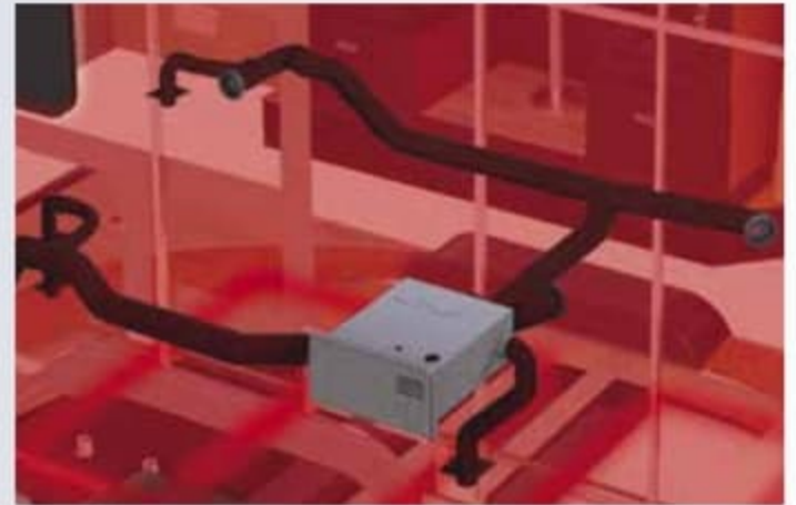
Ducted heat is routed into individually insulated holding tanks to keep them, the valves and PEX lines warm.
