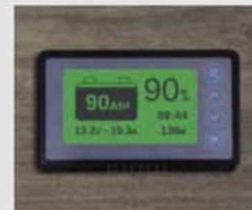
Upgraded battery monitor displays battery statistics like amp-hours consumed, state of charge, and voltage.
