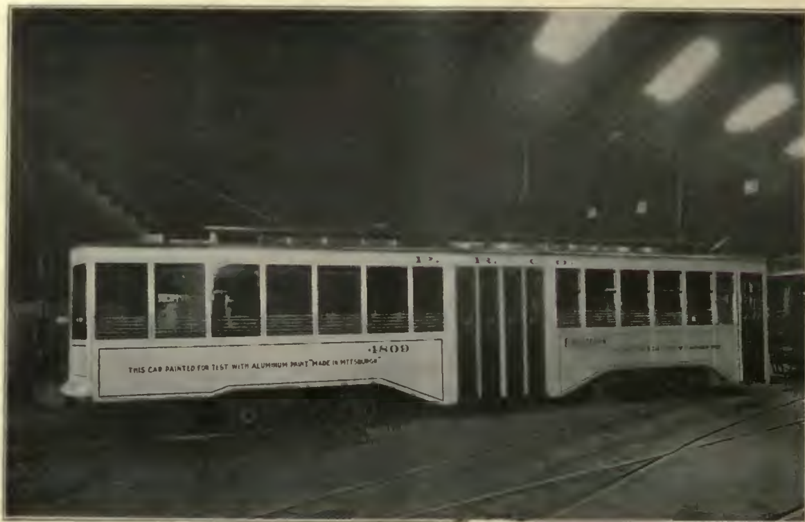
Car of Pittsburgh Railway Company, Pittsburgh, Pa., painted with aluminum paint
