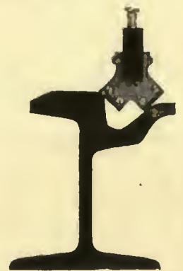
Bar in Place on "Girder" Rail Showing Saw Blade Contacts
