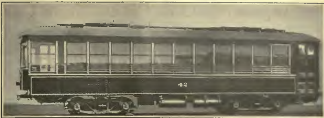
These attractive one-man, double-truck safety cars were delivered to the Helena (Mont.) Light & Railway Co.
