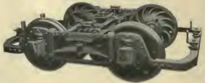
Motor Truck, Class "L," with "Outside Hung" Motors
