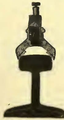
Bar in Place on "T" Rail Showing Saw Blade Contacts
