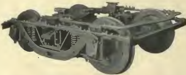
Motor Truck, Class "A," with "Inside Hung" Motors
