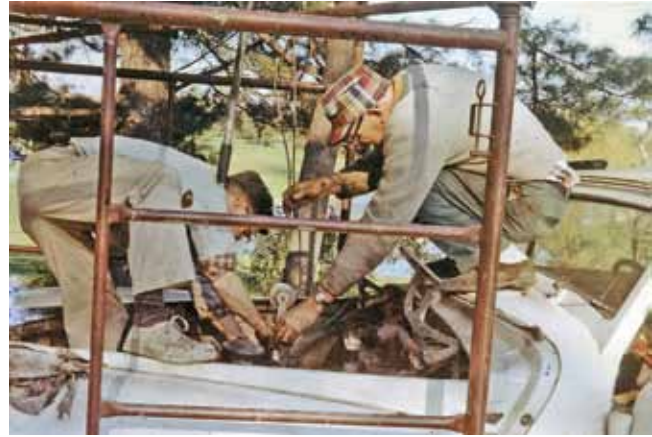
■ Larry Butcher's first Continental project was this Chetwyn Beige 1942 Cabriolet with a postwar grille, no fender skirts, and a smoky Ford V-8 engine. At right, Larry's uncle squats on the cowl to help Larry pull out the old V-8 with a "come-along."
