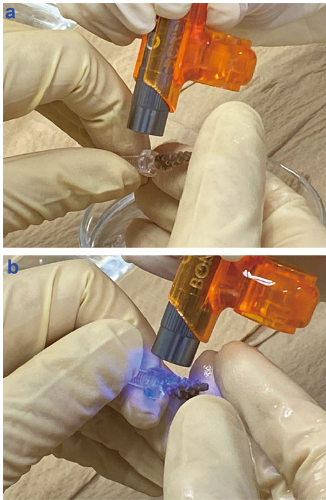
Fig. 8.3 Mounting of coral clone on a polycarbonate bolt using ultraviolet-curable oligomer-based adhesive according to Takeuchi et al. (2019). a Attaching coral clone to the polycarbonate bolt after applying Bondic ® Evo (replaced a pistol grip and new LED from Bondic ® ) to the cut surface of the clone; b Curing of Bondic ® Evo by ultraviolet LED irradiation
