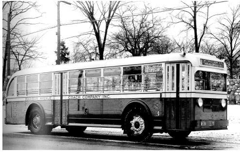
Fig. 12.10 A Yellow Coach with a transverse rear engine, operated by Madison Avenue Coach Inc. in 1934
