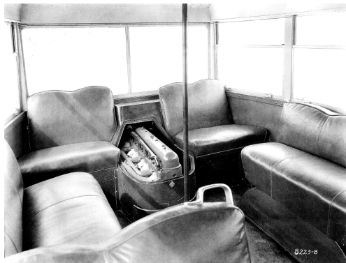
Fig. 12.8 Yellow Coach Company rear-mounted engine, 1933
