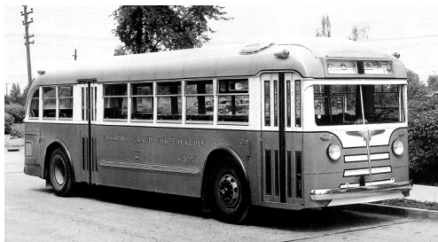
Fig. 12.11 A Yellow Coach with diesel power and monocoque design, operated by Triboro Coach Corporation in 1939
