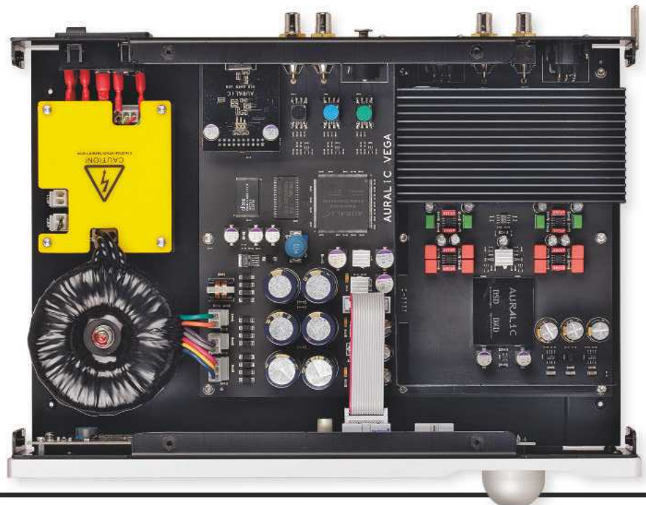
RIGHT: A linear PSU feeds a proprietary LPCM/DXD/DSD-compatible 'Sanctuary Audio Processor' with a claimed '32-bit/1.5MHz' upsampling while an equally bespoke 'Orfeo' Class A analogue stage drives the output
