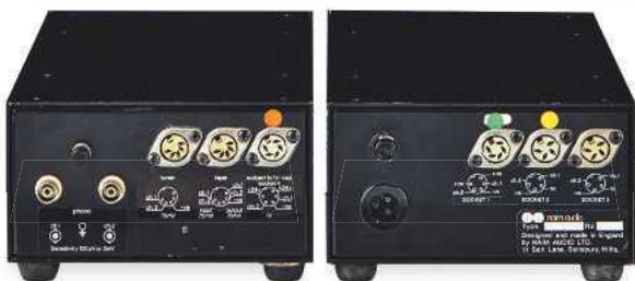
ABOVE: NAP 250 shows XLR signal input (far right) and externally mounted power transistors. Note DIN sockets on NAC 12/SNAPS
