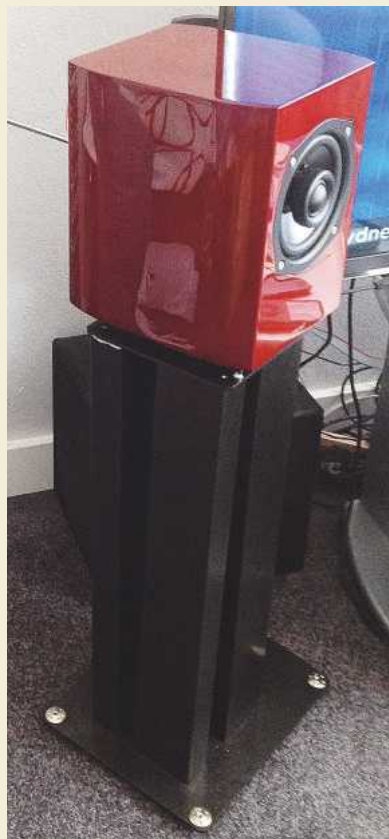
ABOVE: One of Kit's Teac S-300 NEO speakers with its concentric driver array
