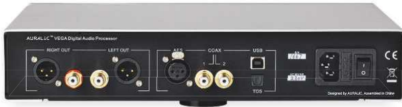
ABOVE: The Vega has five digital inputs: USB, AES/EBU (XLR) and three S/PDIF (two RCA, one Toslink). It has single-ended (RCA) and balanced (XLR) analogue outputs
