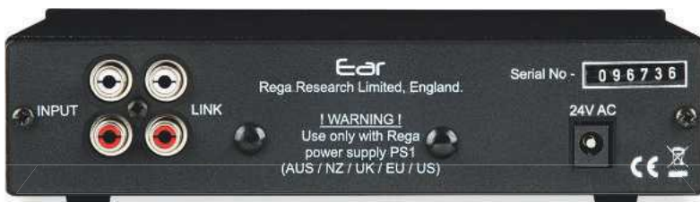
ABOVE: Standard RCA line input and output socketry is all you get on the rear panel of the Rega Ear headphone amplifier, plus the obligatory external power supply input
